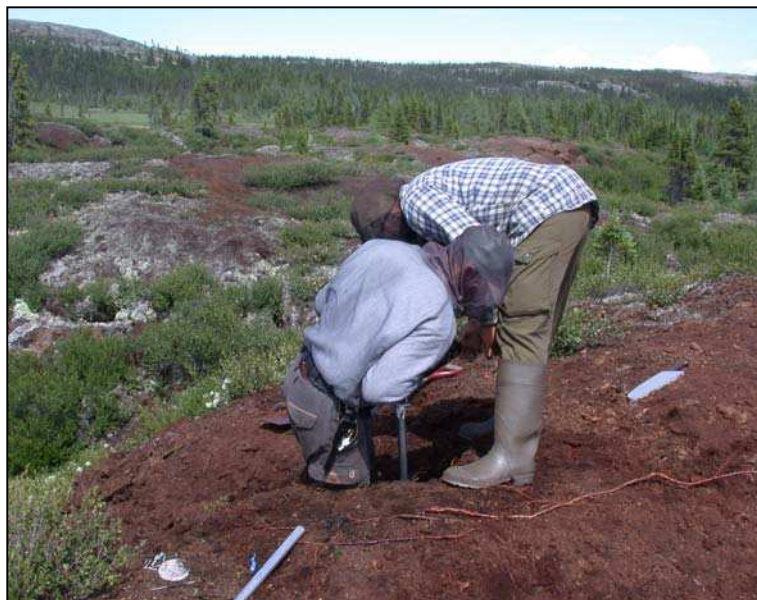
Photo 15. Tommy and Mathieu sampling the palsa bog at site 2 using the Nørnberg corer
