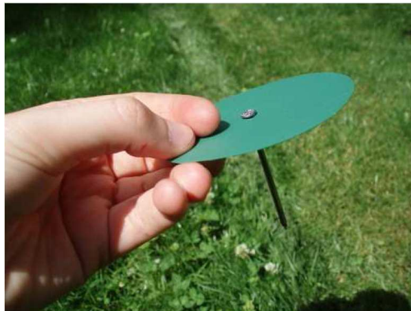
Figure 108: One of the large targets. The nail fixes the target to the ground. The smaller targets are of the same color.
