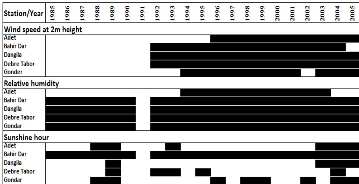
Figure 3-5 Availability of wind speed, relative humidity and sunshine hour data in the Lake Tana basin
