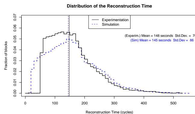
Figure 5.10: Distribution of reconstruction time on a experimentation with 64 nodes during 4 hours compared to simulations.
