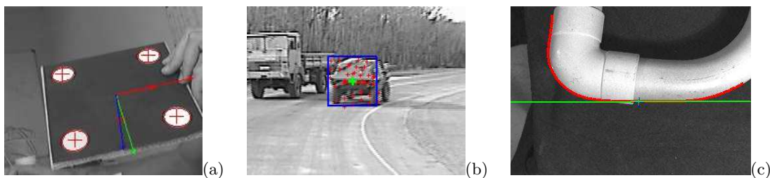
Figure 3.1: Local features are mainly defined by geometrical properties in the image as (a) dots, (b) points of interest and (c) contours.
