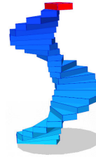
Figure 2.8: Stairs grammar example. On the left the single-rule-shape grammar to make a step. On the right the shape obtained after 25 iterations. The red shape represents the axiom, the blue ones represent the “steps”.
