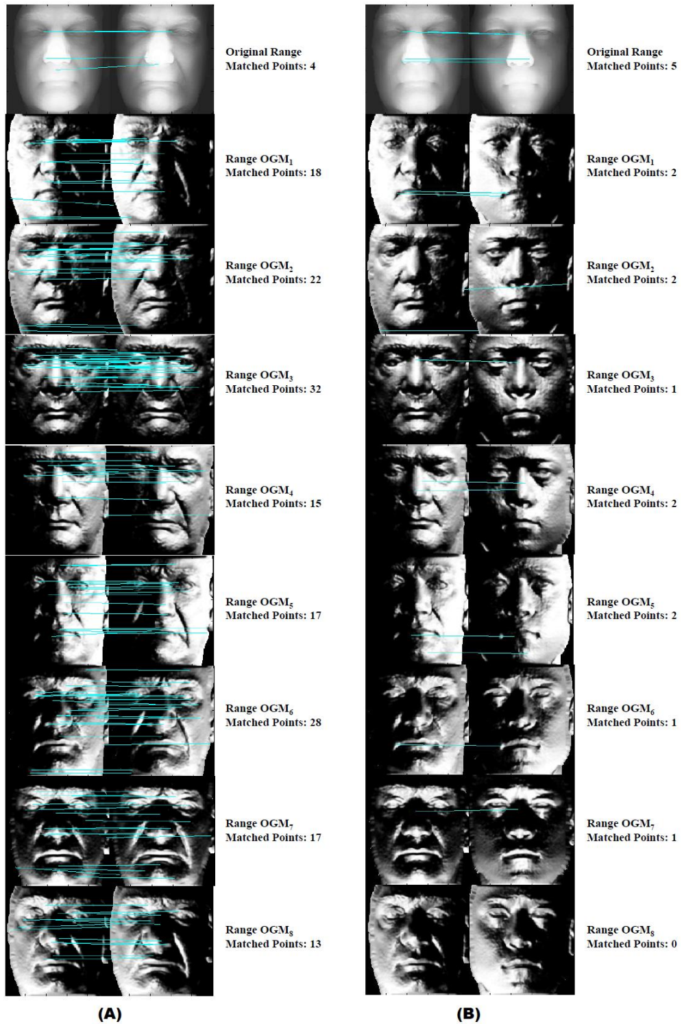
Figure 4.9: Matching examples using original facial range images and their OGMs: (A) matching faces of the same subject; (B) matching faces of different subjects.
