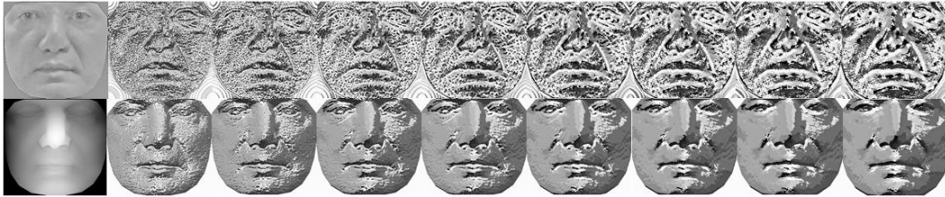
Figure 5.5: LBP faces of facial texture and range images output by the preprocessing pipeline using different neighborhoods: the images from left to right are LBP images generated based on the scale value from 1 to 8 pixels and 8 neighboring points.
