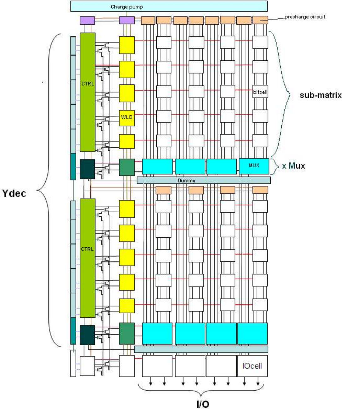
Figure 5.1: Schematic of the 5T-Portless memory cut
