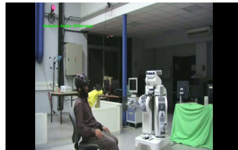
(a) Human Sitting and Looking at the Robot, (b) Human looks away and robot hand is extended CDM selects extend hand action
