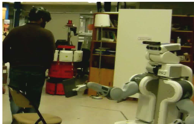
(c) human passes by the robot arm, which is still moving
