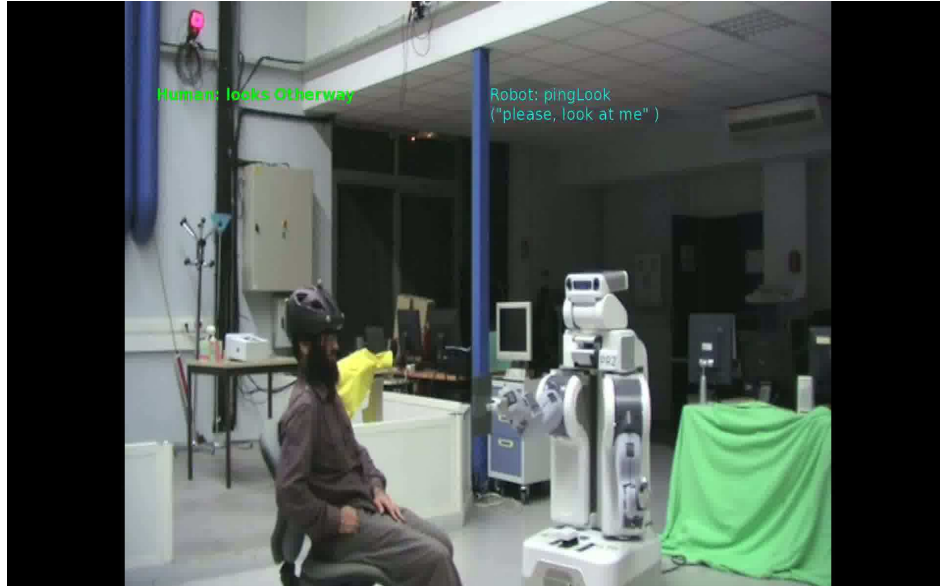
Figure 6.10: PR2 handing over an object to a person, safety issue case (Human lost FoA): This image shows that the human has lost the focus of attention and the robot arm stays extended and the robot asks the human to focus on the task instead of stopping arm motion and moving arm to safe pose.
