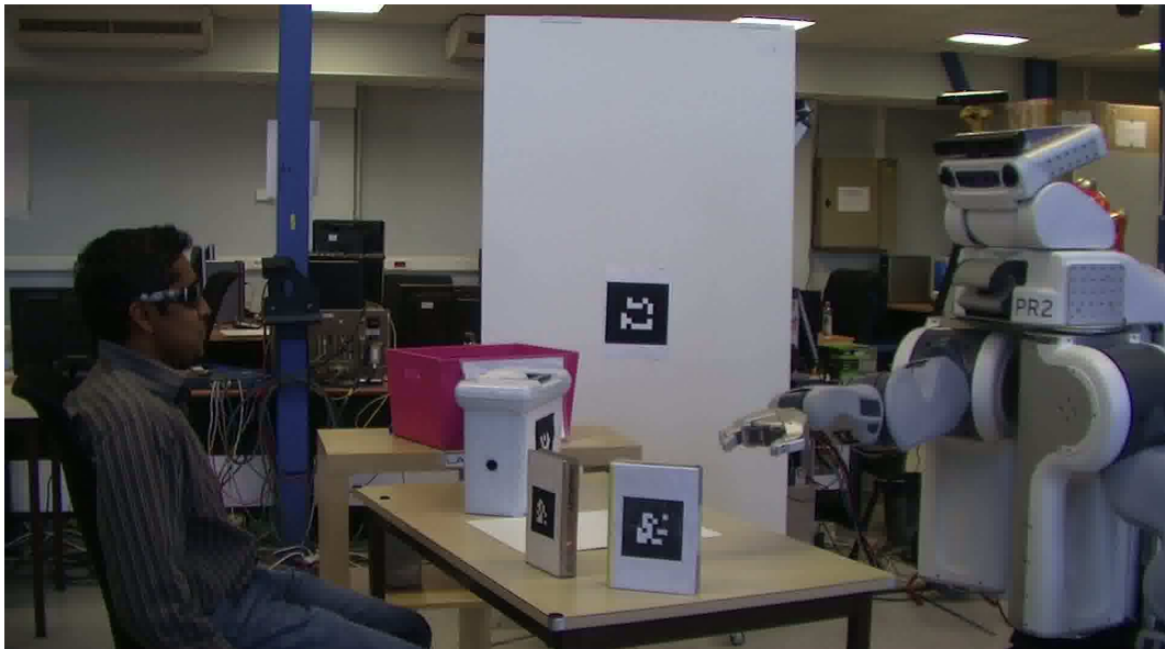
Figure 5.10: Robot proactively moving its arm to ask for human help to get the not reachable object
