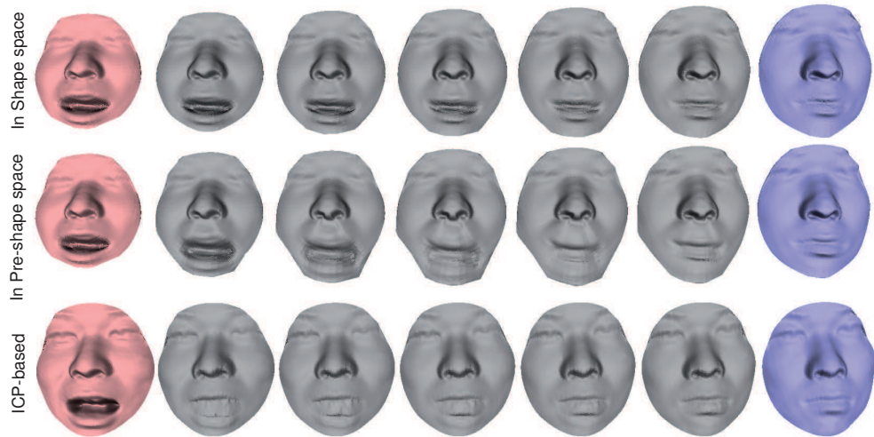
Figure 4.12: Examples of geodesics in shape space, pre-shape space and linearly interpolated path after ICP alignment.
