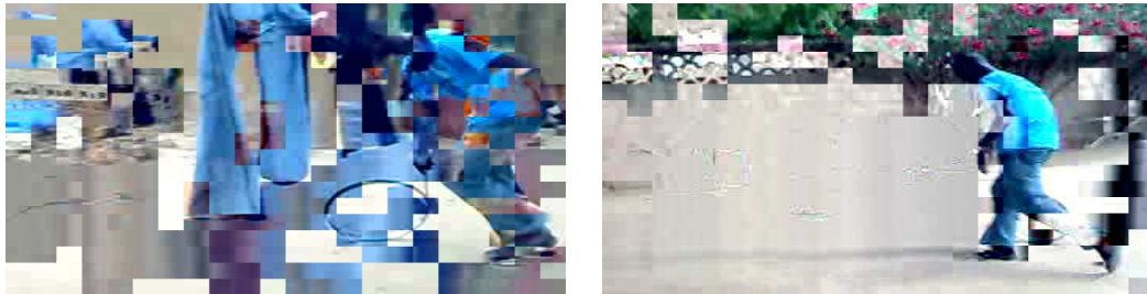
Figure 5.12: Snapshots of the video transmission without QoS (20Mbps background traffic)
