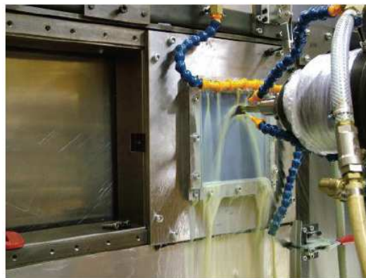
Figure 1.3: Single point incremental sheet forming setup
