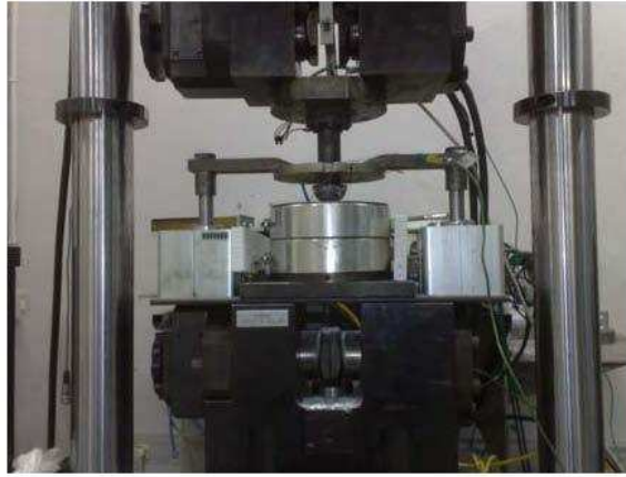
Figure 1.23: Warm Nakazima forming test [64]
