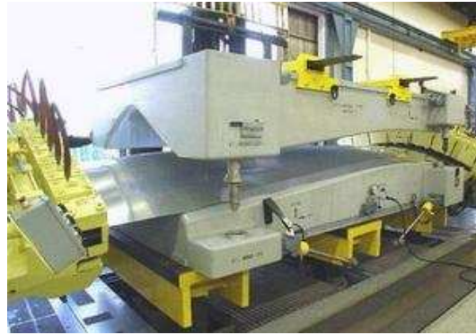
Figure 1.2: Stretch forming process and equipment
