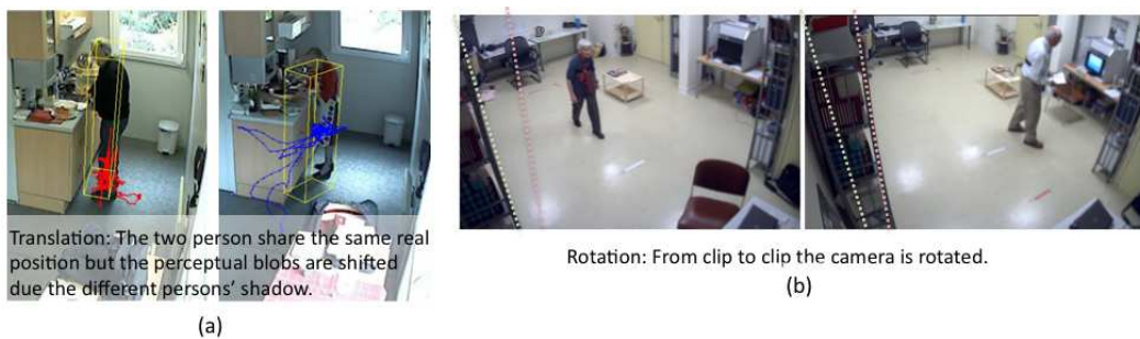
Figure 4.6: Scene alignment problems. a) The blob of the person is shifted due shadows produced by illumination changes, this produces a translation of the SRs of the persons' topology. b) The camera is slightly moved producing a rotation of the persons' topology.
