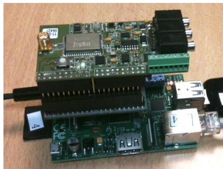
Figure 6-22 Circuit Board of RPiER
