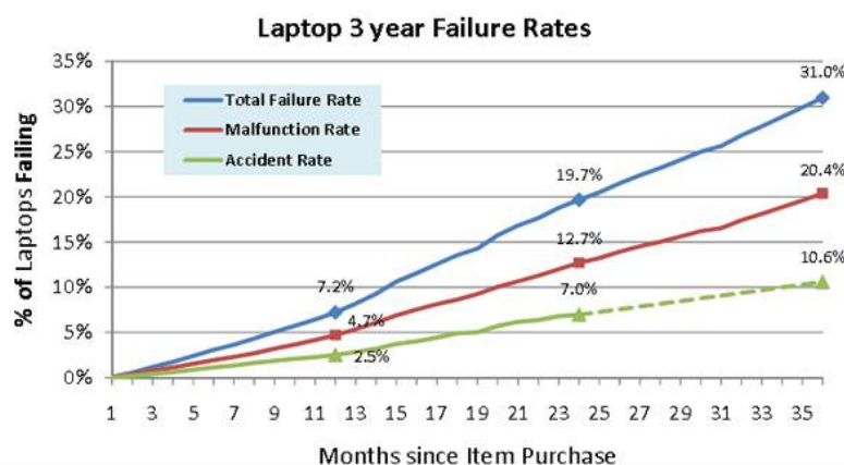
Figure 2-7 Laptop three years Failure Rates (SquareTrade, 2009)
