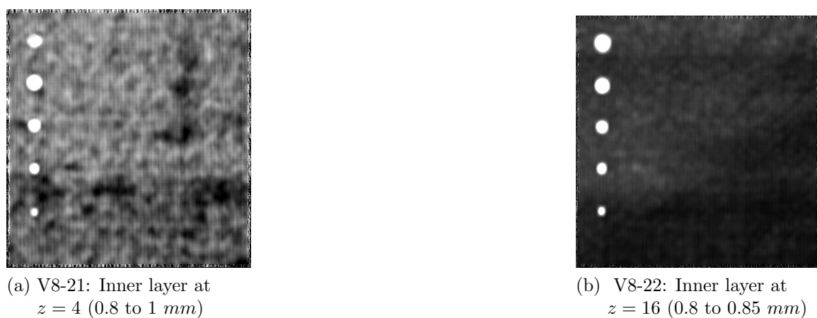
Figure C.5.: Comparison of image quality with SPA technique using different depth resolutions (a) Inner layer of V8-21 at z = 4 . (b) Inner layer of V8-22 at z = 16 .
