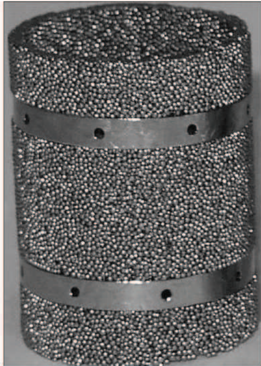
Figure 1. Tracheal prosthesis made of porous titanium with double ring of bulk titanium.
