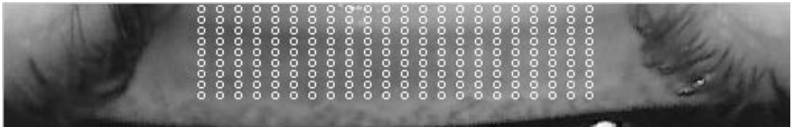
(d) Normalized iris image showing the locations at which the binary features are calculated
