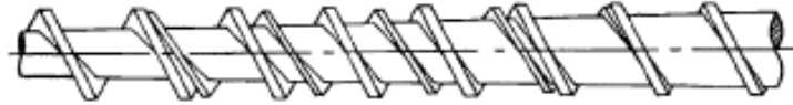
Figure 5 : Profil d'une vis barrière de type "Maillefer", C. Rauwendaal, "Extruder screw with barrier sections", Polymer Engineering and Science , vol. 26, n° 18, page 1245-1253, 1986 [5]
