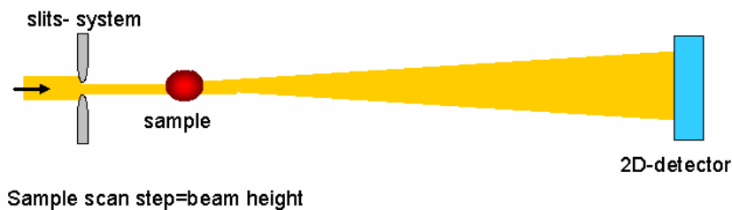
Figure 6.17. Scheme of the experimental set-up used for acquisition with the detector-based analyzer imaging technique.
