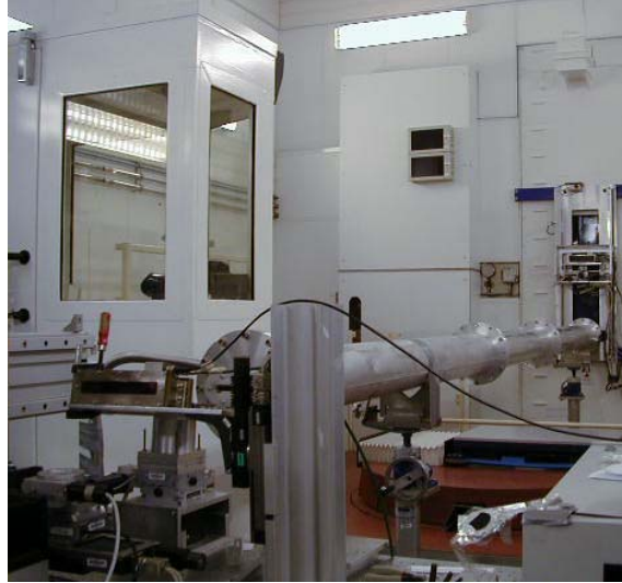
Figure 3.21. The vacuum pipe which is installed in the EH at ID17 when working a low energies (18-30 keV).
