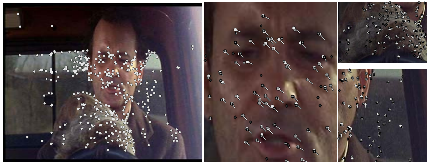
Fig. 3. (left) One frame with points and motion vectors reprojected from the reconstructed model and (right) Closeup on the actor, the groundhog and the background overlaid with points and motion vectors reprojected from the reconstructed model (white dots), original points (light grey squares) and outliers (dark grey diamonds).
