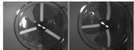
Figure 1. An example of distortion of a rotating ventilator observed with a rolling shutter camera: static object (left image) and moving object (right image).
