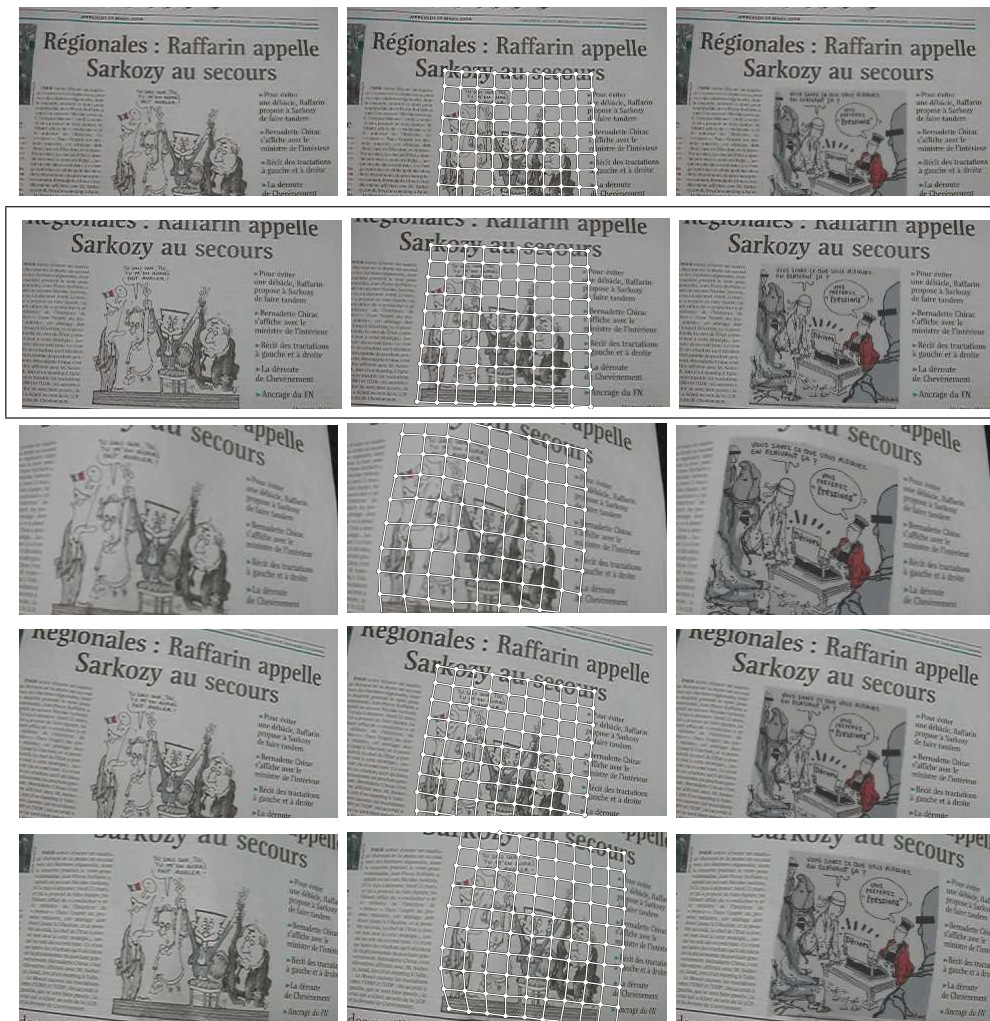
Figure 5: Registration results on the Newspaper sequence. (left) Original images. (middle) A mesh grid illustrating the computed mapping. (right) The cartoon on the reference image (indicated by a black frame) is replaced and mapped onto the other frames.
