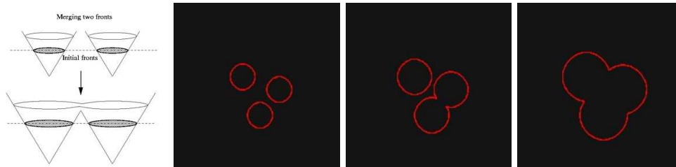
Figure 4.4. Easy handling of contour merging with Level-Sets : \Gamma(x, y, t = 0) is the representation of the three curves. Initializing \phi by the distance to these circles, and propagating \phi with a constant positive speed in the outward normal direction, \phi_t + \beta|\nabla\phi| = 0 , the three circles increase and merge. The different images represent the zero level-set of \phi at several successive iterations.
