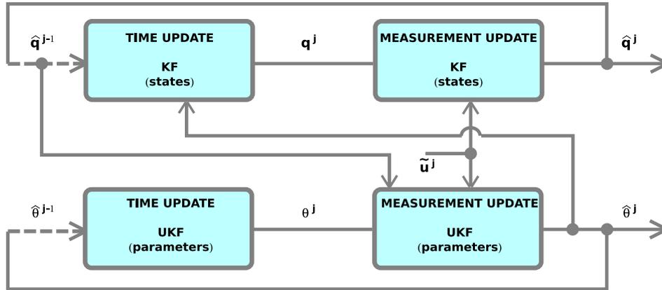
**Figure 4.24:** Block diagram of dual Linear and Unscented Kalman filtering (KF-UKF) for respectively state and parameter estimation.
