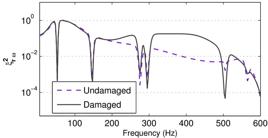
**Figure 4.17:** ECR spectrum for perfect clamped FE model.
