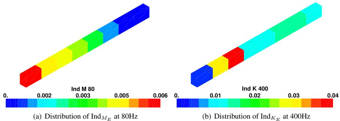
**Figure 4.19:** ECR analysis for a perfect simple-clamped concrete beam FE model. Distribution of most relevant ECR error indicators.
