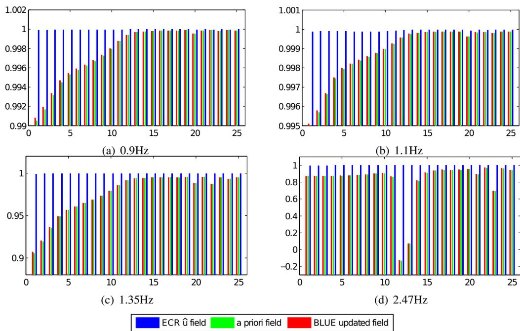
**Figure 4.32:** Sequence of state estimation quality during the damage parameter identification process of a cooling tower example. Comparison of  $\kappa$  criterion between initial guess, ECR and BLUE estimators.
