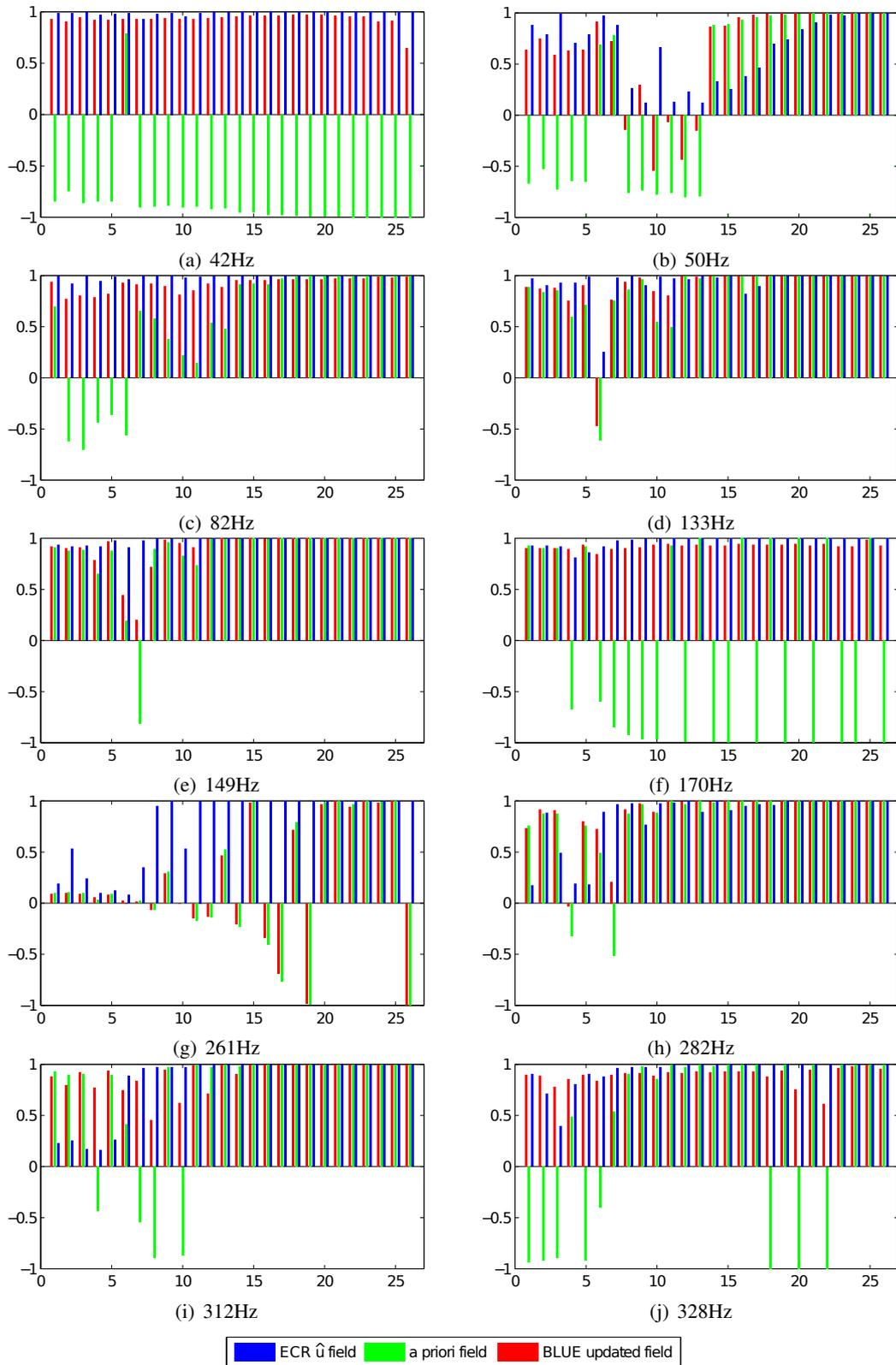
**Figure 4.31:** Sequence of state estimation quality during the damage and boundary impedance parameter identification process of the concrete beam example. Comparison of  $\kappa$  criterion between initial guess, ECR and BLUE estimators.
