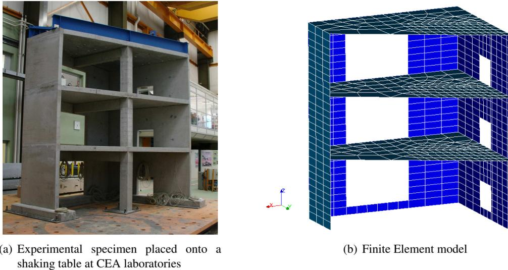
(a) Experimental specimen placed onto a shaking table at CEA laboratories
