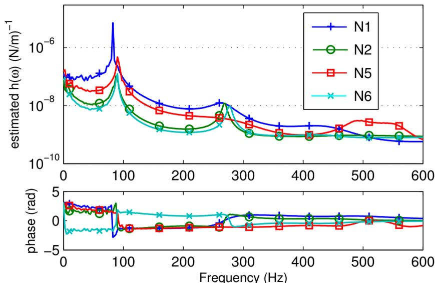
**Figure 4.13:** Identified impedance in  $z$  direction for the erroneous clamping degrees of freedom.
