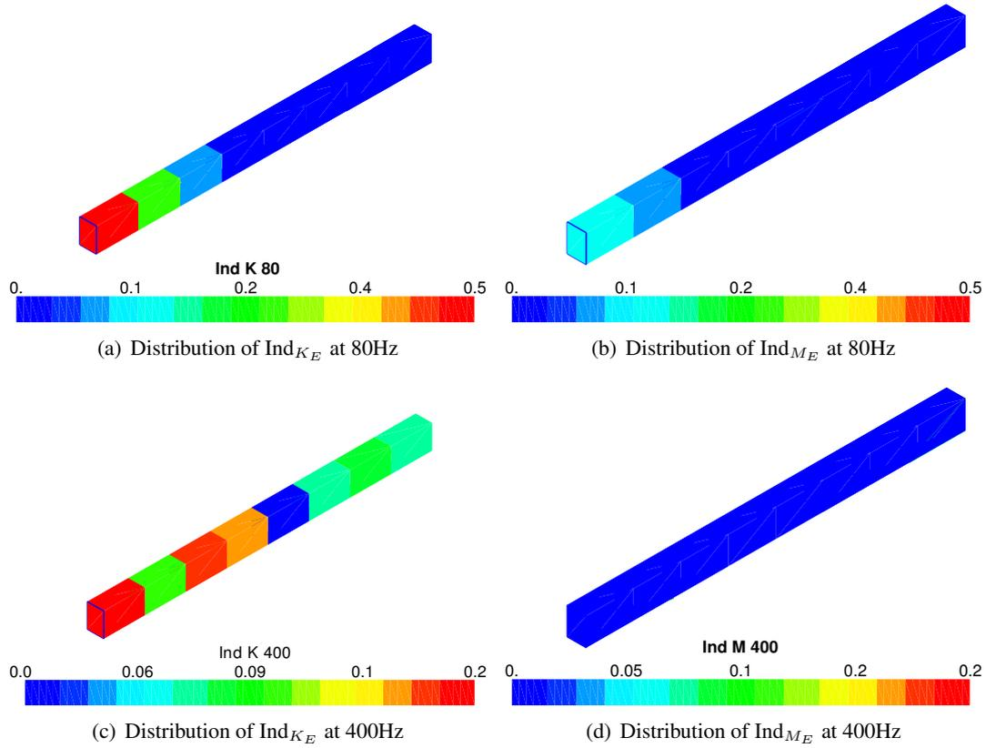
**Figure 4.18:** Preliminary ECR analysis for a perfect double-clamped concrete beam FE model. Distribution of  $IndK$  and  $IndM$  estimators over the structure for different frequencies.
