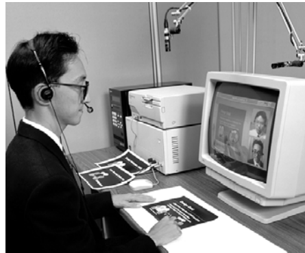
Figure 10. Configuration matérielle de TeamWorkStation (extrait de [Ish99])
