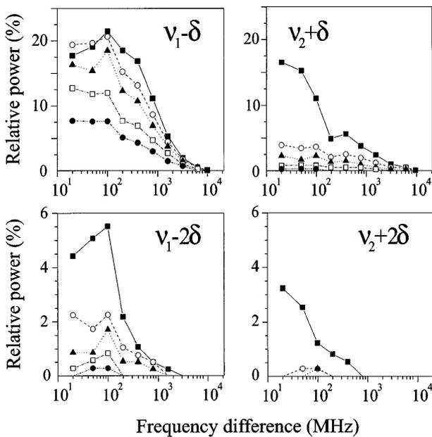
Fig. 4. Fraction of the total power coupled into each sideband at the MOPA output as a function of frequency difference  $\delta$  for different power ratios  $R$  in the injected frequencies. Significant sidebands appear at  $\nu_1 - \delta$ ,  $\nu_2 + \delta$ ,  $\nu_1 - 2\delta$ , and  $\nu_2 + 2\delta$ .<sup>9</sup> Symbols are the same as in Fig. 3.
