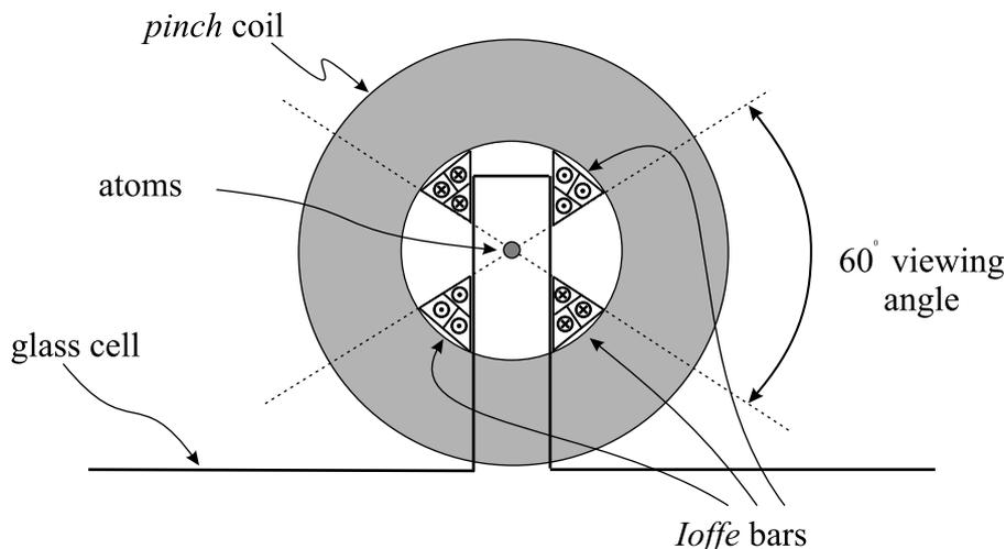
Figure 2.8: Each Ioffe bar consists of three copper tubes. The tubes are deformed to fit in the space between the appendage and the inner surface of the pinch coils, leaving a  $60^\circ$  viewing angle to the atoms.
