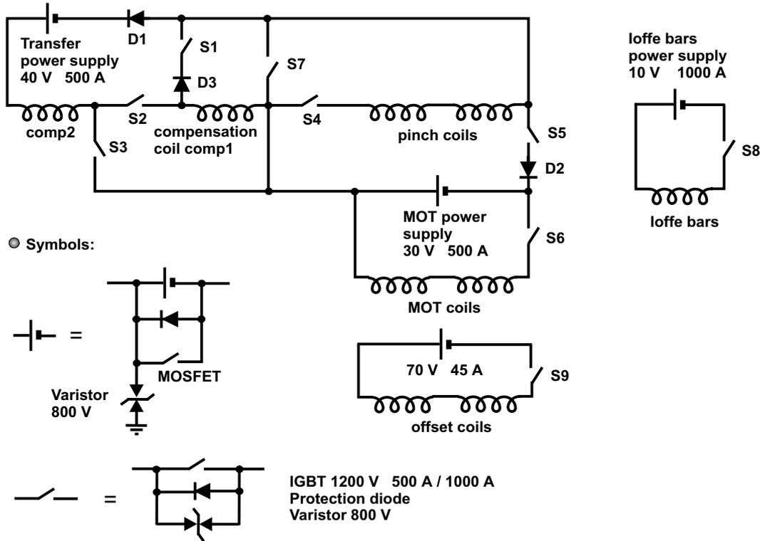
Figure 2.9: *The electric circuit used for the magnetic trap. The power supplies deliver up to 1000 A to the field coils. Different configurations can be achieved using IGBT switches, thus enabling the magnetic transfer of the atoms from the MOT to the appendage region, the reuse of the transfer coils as compensation coils and the use of the pinch or the compensation coils to produce the field necessary for Feshbach resonances. The circuit is explained in detail in the text.*
