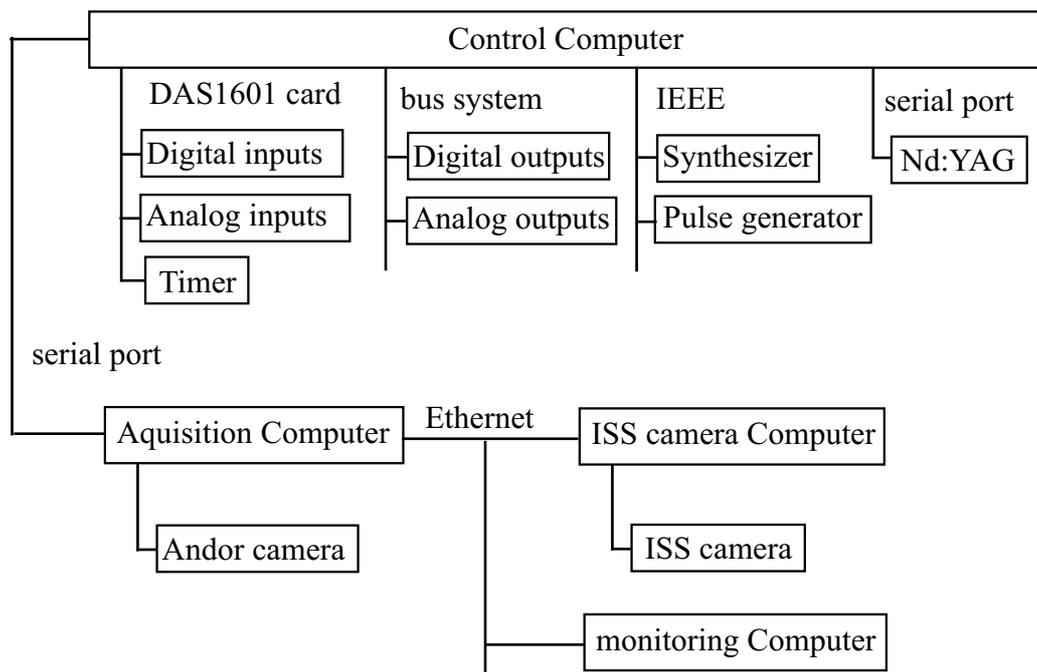
Figure 2.15: *The computer system consists of a control computer and a data acquisition computer. The control computer operates shutters, AOMs, power supplies and so forth by using a digital/analog output system and the IEEE bus and serial ports. It transfers the experimental parameters to the acquisition computer which records, treats and stores absorption images of the atoms.*
