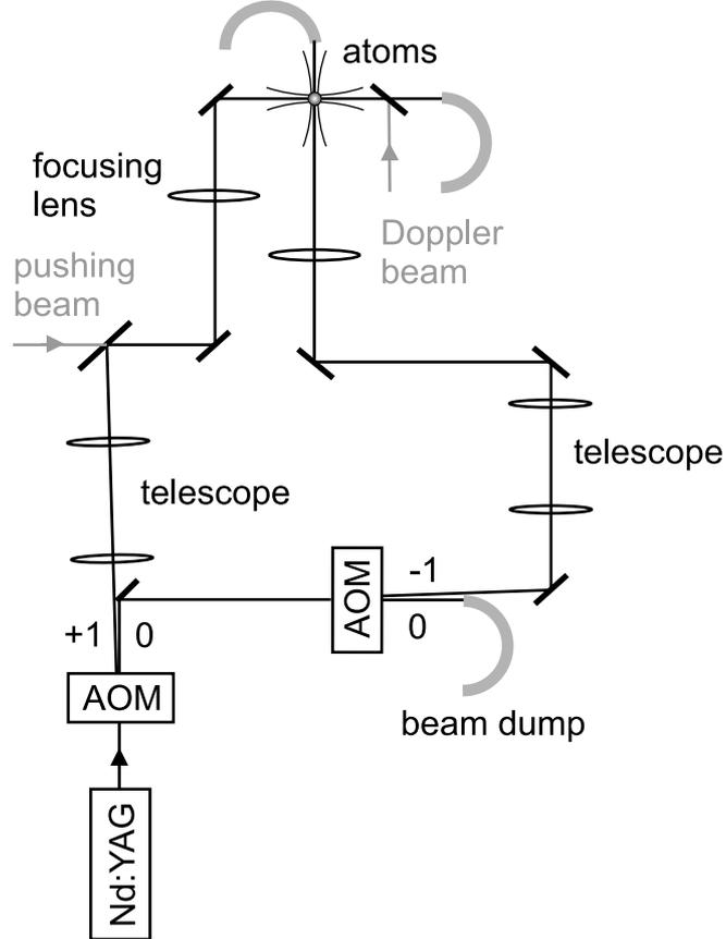
Figure 2.10: *Setup of the crossed optical dipole trap. A 9.5 W Nd:YAG laser beam is split in two beams. They pass through AOMs which are used to control the beam intensities. Both beams are expanded using telescopes and focused under orthogonal directions on the atoms in the Ioffe-Pritchard trap region. The 671 nm pushing beam and the Doppler cooling beam are coupled into the horizontal dipole trap beam by using dichroic mirrors.*
