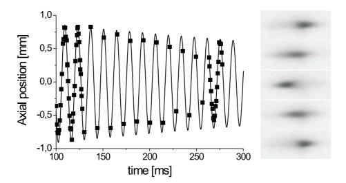
Figure 3.8: Determination of the axial oscillation frequency. The atomic cloud is pushed out of its equilibrium position using the Doppler cooling beam. After a sudden switch off of the beam, the cloud oscillates in the trapping potential. In this example the oscillation frequency is  $\omega_{ax} = 2\pi \times 72 \text{ Hz}$ .
