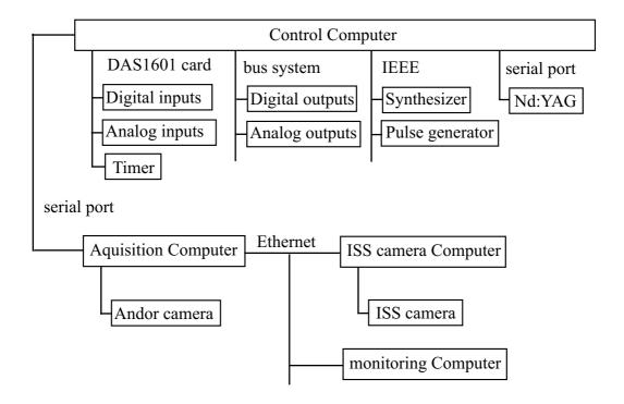
Figure 2.15: The computer system consists of a control computer and a data aquisition computer. The control computer operates shutters, AOMs, power supplies and so forth by using a digital/analog output system and the IEEE bus and serial ports. It transfers the experimental parameters to the aquisition computer which records, treats and stores absorption images of the atoms.
