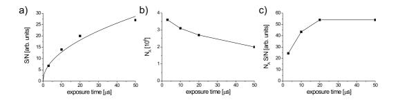
Figure 2.14: Optimization of the detection system. Signal to noise ratio S/N (a), measured atom number  $N_A$  (b) and  $N_A S/N$  plotted versus the exposure time.
