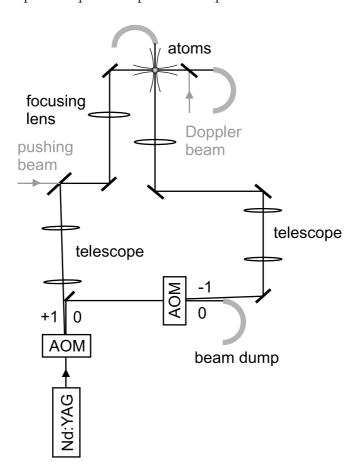
Figure 2.10: Setup of the crossed optical dipole trap. A 9.5 W Nd:YAG laser beam is split in two beams. They pass through AOMs which are used to control the beam intensities. Both beams are expanded using telescopes and focused under orthogonal directions on the atoms in the Ioffe-Pritchard trap region. The 671 nm pushing beam and the Doppler cooling beam are coupled into the horizontal dipole trap beam by using dichroic mirrors.
