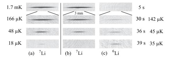
Figure 3.18: Images of <sup>6</sup>Li and <sup>7</sup>Li atom clouds at various stages of sympathetic cooling (b,c) and during single-species evaporation (a) with identical initial numbers of <sup>7</sup>Li atoms. Top images are 1 cm long, the others 3 mm. Temperatures of <sup>7</sup>Li (resp. <sup>6</sup>Li alone) are given on the left (right).
