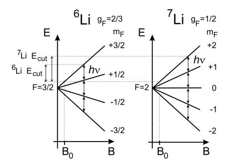
Figure 3.13: Zeeman radio frequency transition in the higher hyperfine states. Shown is the magnetic field dependence of the  $m_F$  substates of  $^6Li$  and  $^7Li$  for weak magnetic fields.  $B_0$  is the offset magnetic field of the trap. A radio frequency wave with frequency  $\nu$  corresponds to a lower cut energy  $E_{cut}$  for  $^6Li$  than for  $^7Li$ . This makes sympathetic cooling of  $^6Li$  by  $^7Li$  with a Zeeman transition impossible.
