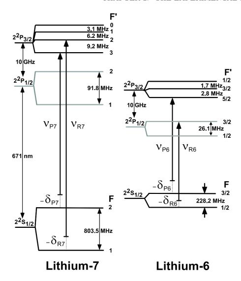
Figure 2.4: Energy level diagram for the lower S and P levels of  $^7Li$  and  $^6Li$ . The transitions used for the MOT are shown, the index P referring to the principal transition and the index R to the repumping transition. Note that  $^6Li$  is repumped on the D1  $(2^2S_{1/2} \Rightarrow 2^2P_{1/2})$  transition since the D2  $(2^2S_{1/2} \Rightarrow 2^2P_{3/2})$  repumping transition coincides with the D1 transition of  $^7Li$ .
