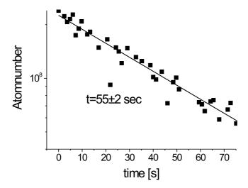
Figure 3.12: Background gas collision limited lifetime of a gas after Doppler cooling. The gas is stored in a trap with oscillation frequencies of  $\omega_{ax} = 2\pi \times 73$  Hz and  $\omega_{rad} = 2\pi \times 200$  Hz and an offset magnetic field of 480 G. The lifetime is 55(2) s. The best observed lifetime under these conditions has been 140 s, due to a lower background gas pressure.
