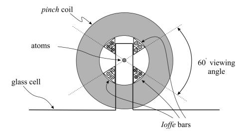
Figure 2.8: Each Ioffe bar consists of three copper tubes. The tubes are deformed to fit in the space between the appendage and the inner surface of the pinch coils, leaving a 60° viewing angle to the atoms.
