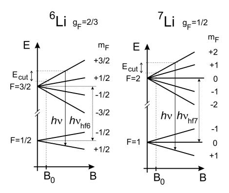
Figure 3.14: Evaporation on the hyperfine transition of  $^6Li$  and  $^7Li$ . Due to the difference in the hyperfine splitting  $\nu_{hf6} = 228.205 \, MHz$  and  $\nu_{hf7} = 803.504 \, MHz$  of the two isotopes the evaporation is isotope selective.  $B_0$  indicates the offset magnetic field of the trap.
