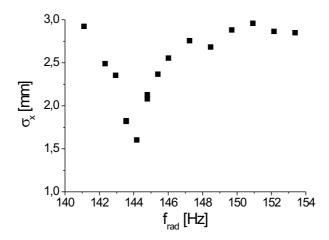
Figure 3.9: Cross dimensional rethermalization. A cloud with higher axial than radial temperature is prepared. After a delay of 400 ms, the axial size is measured. A strong reduction in the axial size is observed if the radial oscillation frequency is the double of the axial frequency. Here the axial oscillation frequency was measured as shown in figure (3.8) and is 72 Hz.
