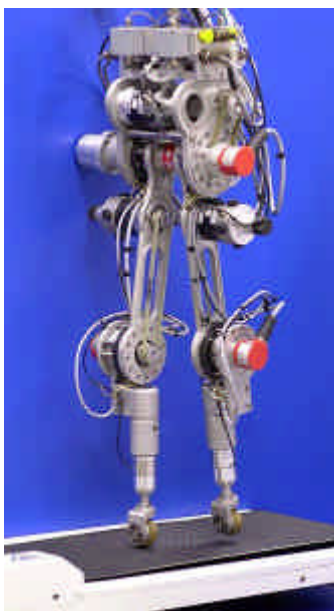
Figure III–8. Robot bipède RABBIT.
