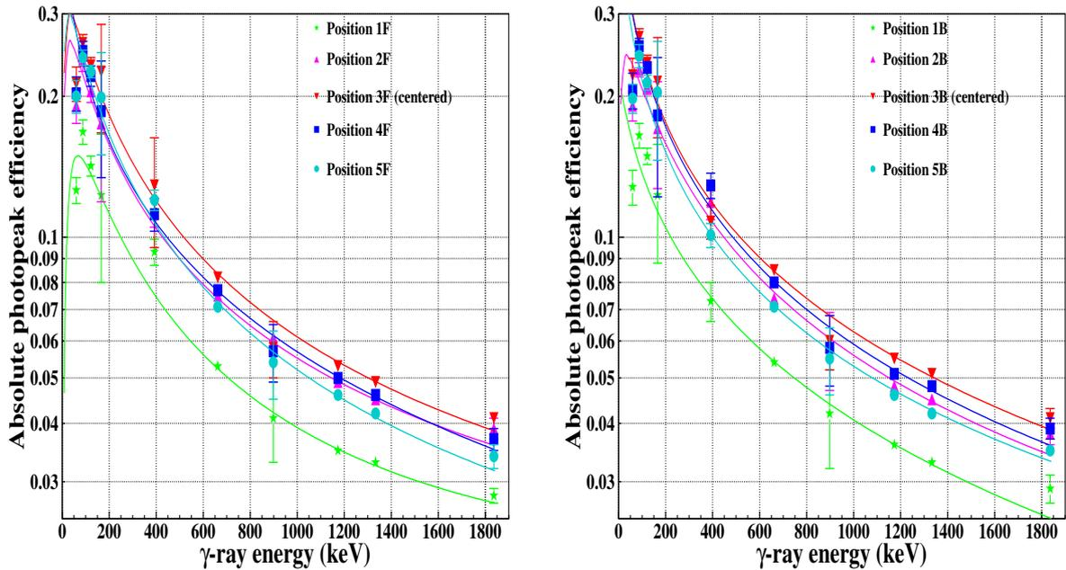
Figure 3.6: Results of the photopeak efficiency calibration of the Segmented Clover array. The right graph corresponds to calibration with the source on the side where the beam is entering the catcher. The left graph corresponds to calibration with the source on the side where the beam would leave the catcher. More details about source positions are given in figure 2.9.
