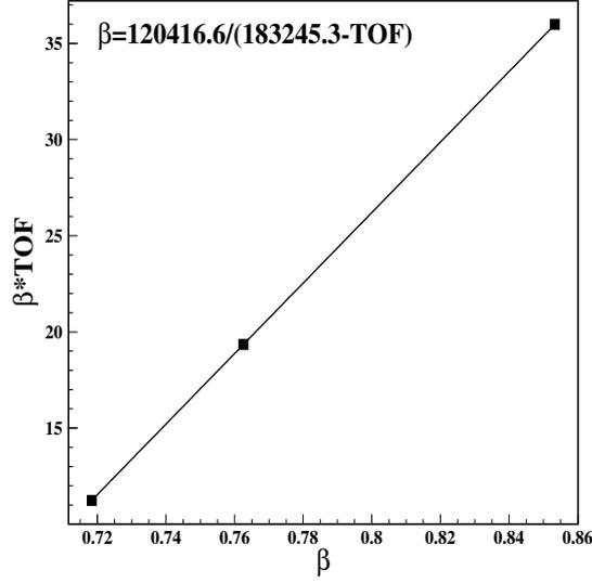
Figure 3.1: Determination of the velocity as a function of TOF. The fit function is deduced from the linear fit of  $\beta \cdot TOF$  as a function of  $\beta$ . The three calibration points correspond to three different thicknesses of the S2 degrader.
