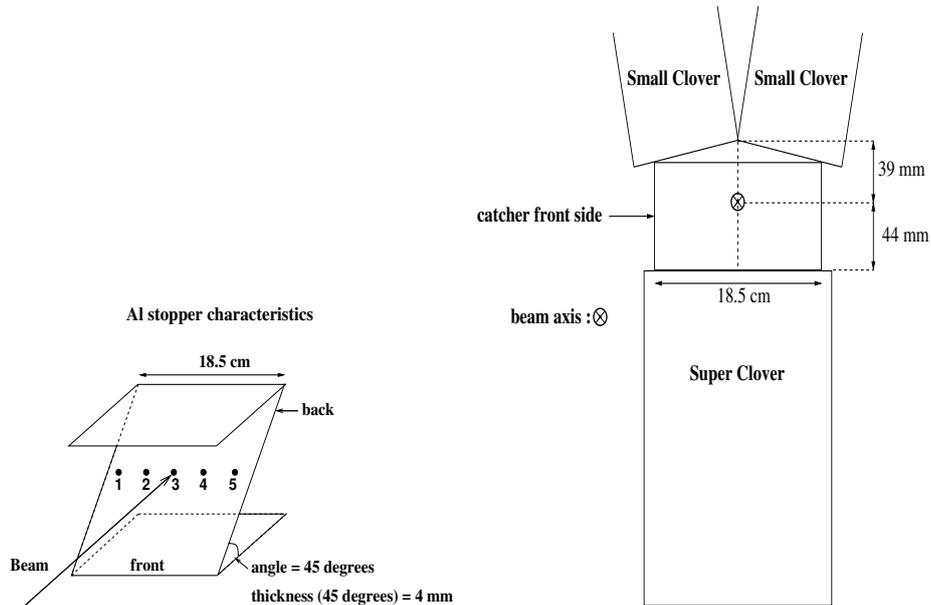
Figure 2.9: Characteristics of the stopper and scheme of the Clovers set-up.
