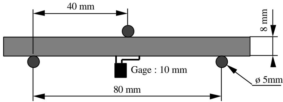
Fig.13 The 3-point bending tests.
