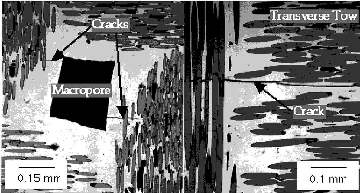
Fig.4 Micrograph showing examples of cracks initiated at a macropore (first family) and cracks initiated in the transverse tow (second family) in a SiC/SiC composite subject to tensile loading [Gui94].
