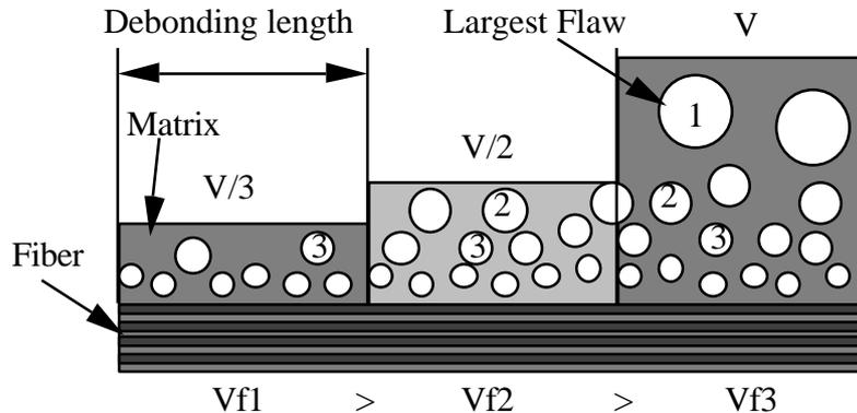
Fig.16 Flaw size dependence with fibre volume fraction  $V_f$ .
