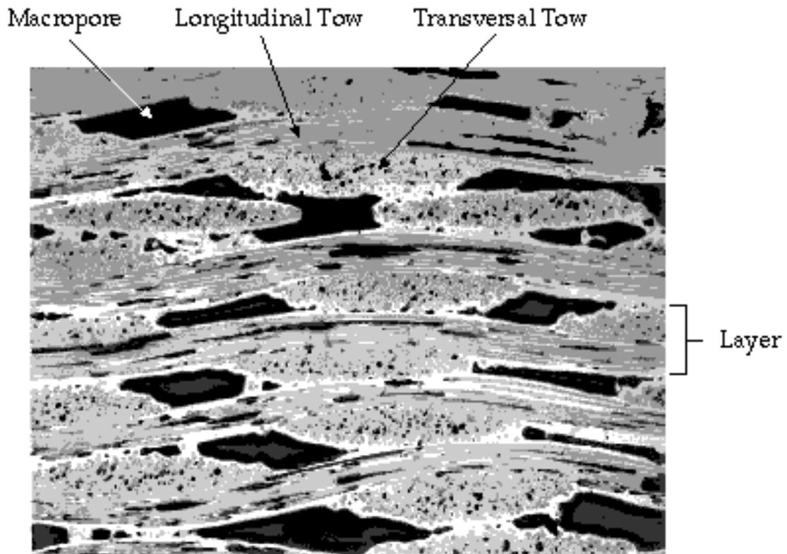
Fig.2 Structure of a woven SiC/SiC composite [Gui94].
