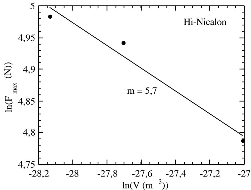
Fig.4 Scale effect on bundle ultimate failure loads for various fibre volumes (lengths).
