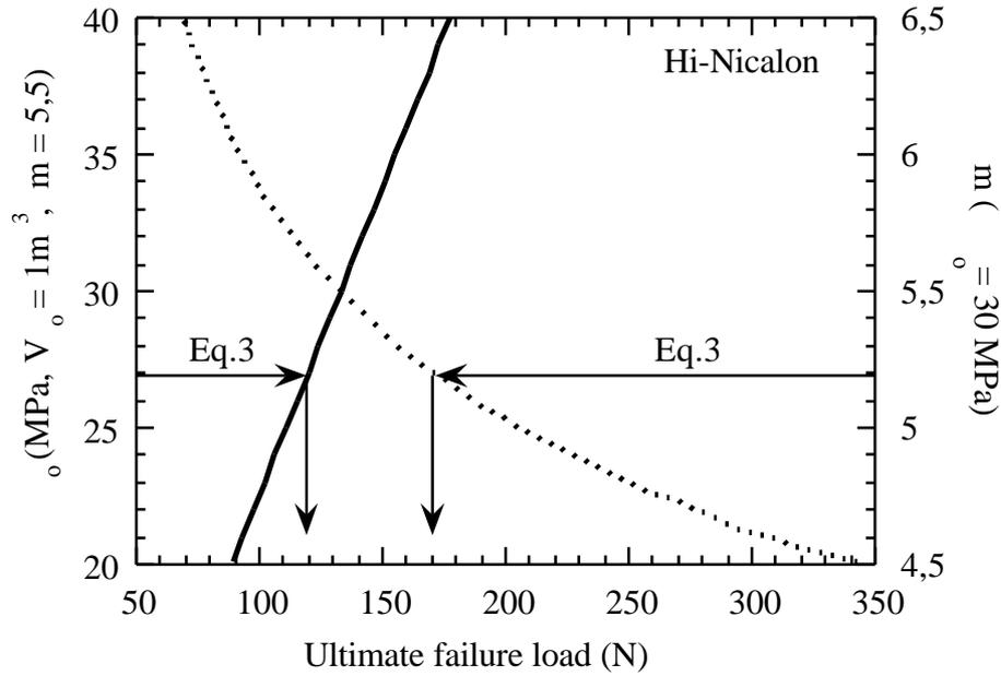
Fig.3  $m$  and  $\sigma_0$  influence on the ultimate failure load (Solid line : the ultimate load is a linear function of  $\sigma_0$  with  $m=5.5$ ) (Dotted curve : the ultimate load follows an exponential curve of  $m$  with  $\sigma_0=30\text{MPa}$ ).
