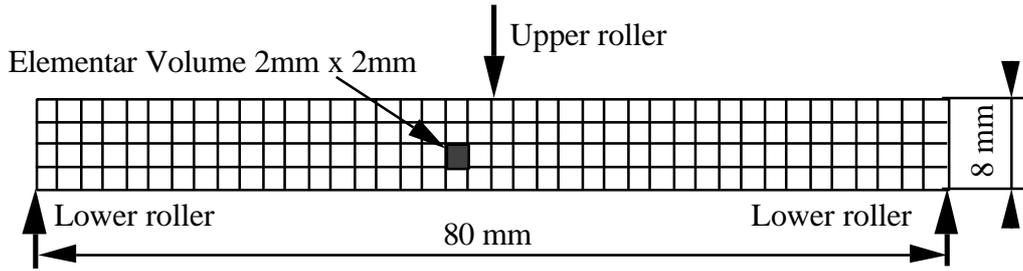
Fig.4 Example of a bending specimen (8mm x 80mm x 3,3mm) with 4 x 40 elementary volumes (Woven SiC/SiC composite).
