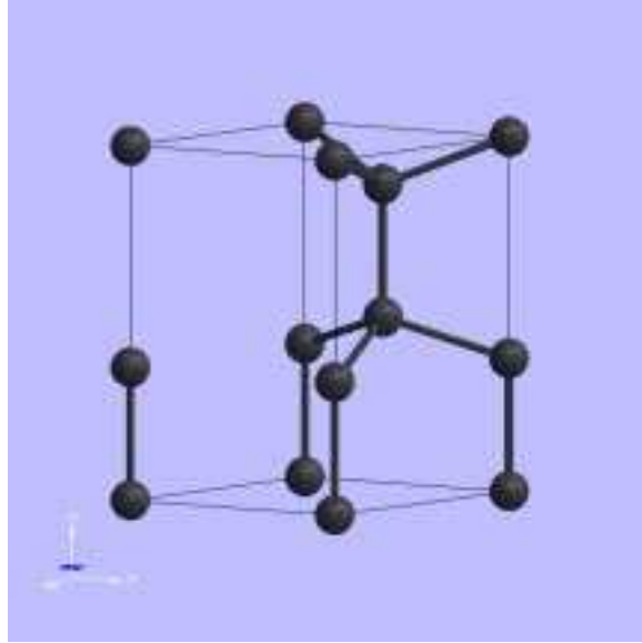
Figure 9.2: Unit cell of lonsdaleite (hexagonal polymorph of diamond).
