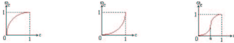
Figure 3.34. Examples of stretching functions: (a) Privileges small values of the cost; (b) penalizes small values of the cost; (c) penalizes values of the cost below a and favors values of the cost above a .
