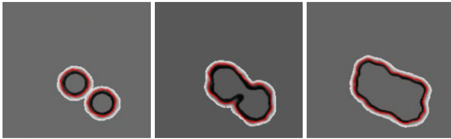
Figure 5.8. Narrow Band reconstruction: images are samples of the evolution and reconstruction of the narrow-band, starting from two circles that merge.
