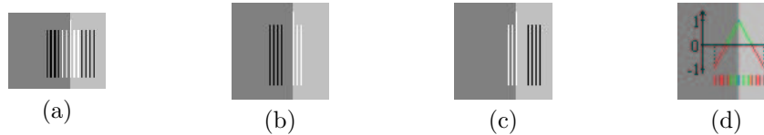
Figure 3.31. Training areas: In white the positive area and in black the negative one. The longest line is the training path. (a) Symmetric. (b) Asymmetric for inside feature. (c) Asymmetric for outside feature. (d) Schematic weighting function.
