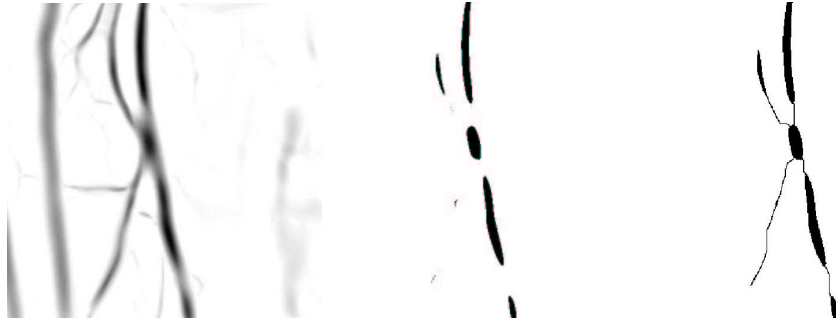
Figure 9.21. Perceptual Grouping on a 2D Medical Image: left image is the vesselness potential; middle and right images show that from the set of regions obtained from thresholding of potential image, our method finds links between these regions as minimal paths with respect to the potential.
