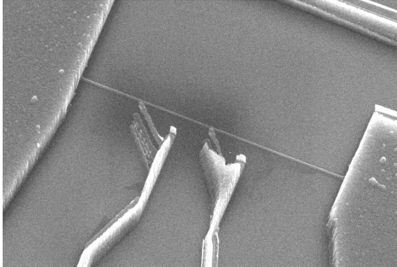
Figure 8: SEM micrograph of the sample viewed at an angle of  $40^\circ$ . The 120 nm-wide, 10  $\mu\text{m}$ -long superconducting wire is connected to large superconducting thick pads. Two normal probes form tunnel junctions with the wire in order to measure the density of states in the superconducting wire.
