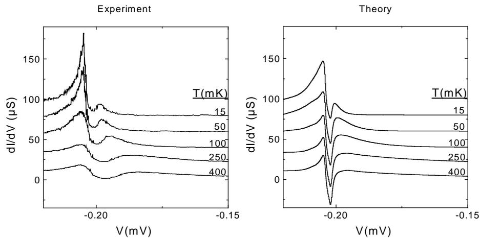
Figure 9: Measured and calculated differential conductance of the side tunnel junction as a function of the temperature when a supercurrent of 9 nA flows in the wire. Assuming that the superconducting pads are not modified, only the filling of the states in the normal wire is modified. When the temperature increases, the same evolution is found qualitatively.
