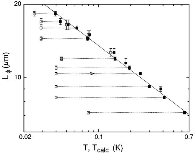
FIG. 11. Full symbols: phase coherence length measured on a 6N silver sample as a function of the electronic temperature  $T_{\text{calc}}$  calculated using Eq. (A2) for a cryostat temperature  $T$  represented by the attached open symbol. The continuous line represents the theoretical prediction  $L_\phi \propto T^{-1/3}$  of electron–electron interactions (data taken at Saclay).
