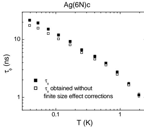
Figure 3: Phase coherence time  $\tau_\phi$  versus temperature in the sample Ag(6N)c (see paper below). Open symbols: Phase coherence time obtained by fitting the magnetoresistance data with Eq. (5). Full symbols: Phase coherence time obtained when taking into account effect of the finite length of the wire using Eq.(9).
