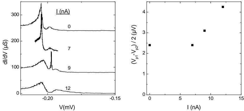
Figure 10: Left panel: Differential conductance of the side tunnel junction when the wire carries a supercurrent. A minigap opens in the wire density of states, leading to the peak near the gap edge of the superconducting electrode. Right panel: Difference between the positions  $V_{p1} - V_{p2}$  of the peaks in the differential conductance versus the supercurrent.
