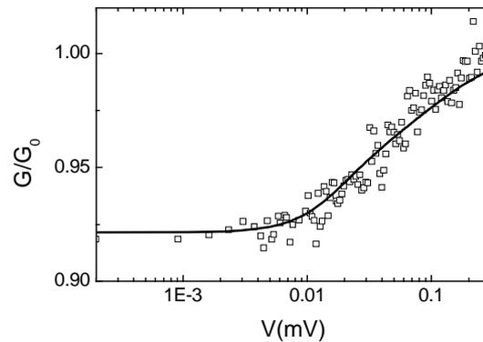
Figure 9: Differential conductance of the tunnel junction between the side probe electrode and the wire in its normal state, normalized to the conductance  $G_0$  at large voltage. Due to Coulomb blockade, the conductance presents a dip at low voltage. The line is a fit using Coulomb blockade theory (Eqs. (19) and (20)) with an electromagnetic environment that consists of the parallel combination of  $R_{eff} = 250 \Omega$  and  $C_{eff} = 8 \text{ fF}$ .
