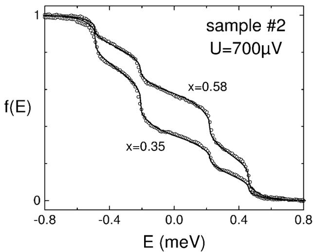
FIG. 3. Distribution functions on sample No. 2, at two positions ( $x \equiv X/L = 0.58$  and  $x = 0.35$ ), for  $U = 700 \mu\text{V}$ . Symbols: experiment. Solid lines: solution of the Boltzmann equation accounting for the Andreev reflections at the reservoirs and electron-electron interactions within the wire.
