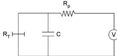
Figure 5: Electrical circuit representing a tunnel junction in a resistive environment: the junction between the wire and the probe is decomposed into a tunnel element of resistance  $R_T$  in parallel with a capacitance  $C$ , whereas the probe electrode is represented as a resistance  $R_p$ . The environment impedance  $Z(\omega)$  is the parallel combination of  $R_p$  and  $C$ .
