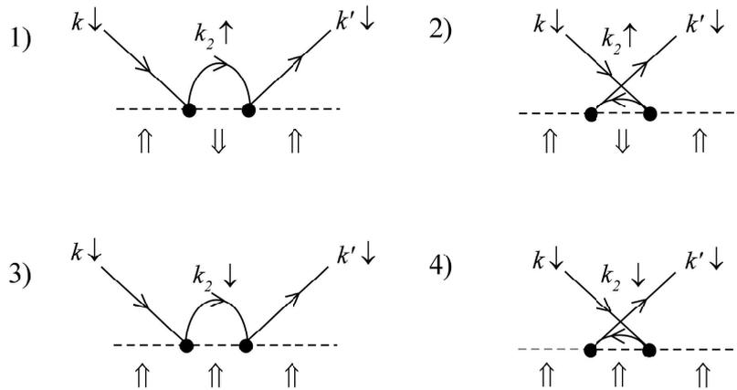
Figure 3: First and second order elastic processes involving one electron and one magnetic impurity in a case where initial and final electron spin states are identical.
