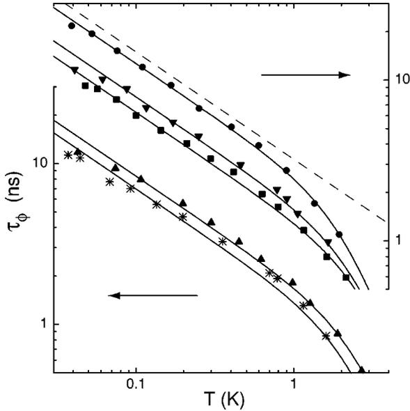
FIG. 4. Phase coherence time vs temperature in samples Ag(6N)a (■), Ag(6N)b (▼), Ag(6N)c (●), Ag(6N)d (▲), and Au(6N) (\*), all made of 6N sources. Continuous lines are fits of the data to Eq. (4). For clarity, the graph has been split in two part, shifted vertically one with respect to the other. The quantitative prediction of Eq. (3) for electron–electron interactions in sample Ag(6N)c is shown as a dashed line.
