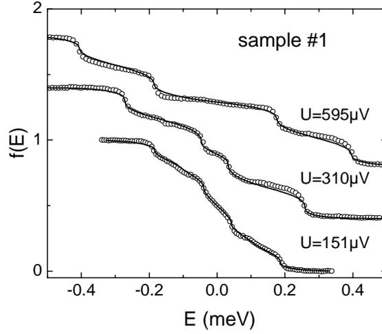
Figure 16: Energy distribution function in the middle of the wire of sample 1, when the reservoirs are in the superconducting state and voltage biased at  $U$ . Symbols are experimental data; solid lines are the solution of the Boltzmann equation taking into account multiple Andreev reflections and energy exchange.
