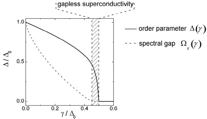
Figure 3: Order parameter  $\Delta(\gamma)$  and spectral gap  $\Omega_g(\gamma)$  in units of the order parameter  $\Delta_0$  at  $B=0$  and  $I_S=0$  versus depairing energy. When  $0.45\Delta_0 \leq \gamma \leq 0.5\Delta_0$ , gapless superconductivity occurs. When  $\gamma \geq 0.5\Delta_0$ , superconductivity is suppressed.
