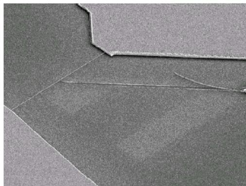
Figure 3: One-step fabrication of a sample for the energy exchange measurement in a magnetic field. Top: exposure pattern of the center of the chip, with dose encoded in levels of gray. The arrows indicate schematically the order and angle of deposition of the different metals. Bottom: Actual sample, seen at an angle.
