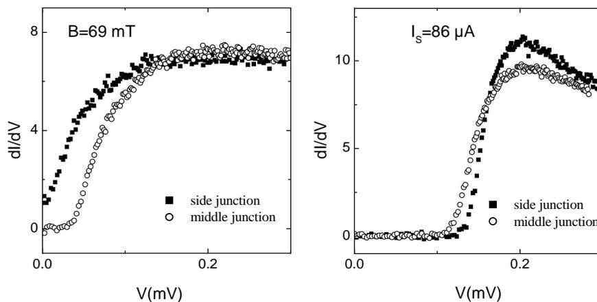
Figure 15: Comparison of differential conductances of the two probe tunnel junctions at  $B = 69$  mT and  $I_s = 0$  (left panel) and  $B = 0$  and  $I_s = 86 \mu\text{A}$  (right panel). At the position of the side junction, the magnetic field induces more depairing whereas supercurrent induces less depairing than at the middle junction. This difference is explained by the different widths of the wire at the two junctions. At the position of the side junction, the wire is wider.
