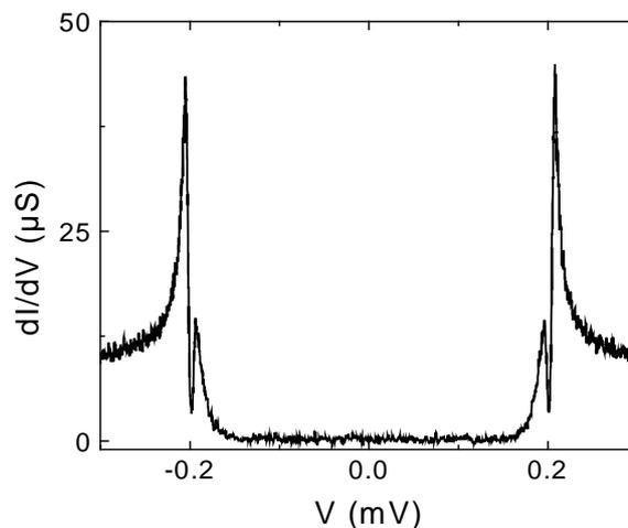
Figure 7: Differential conductance  $dI/dV$  of the side tunnel junction when the normal wire sustains a supercurrent  $I_s = 9$  nA. Additional structures appear near the gap of the probe electrode  $\Delta_p = 200\mu\text{V}$ .
