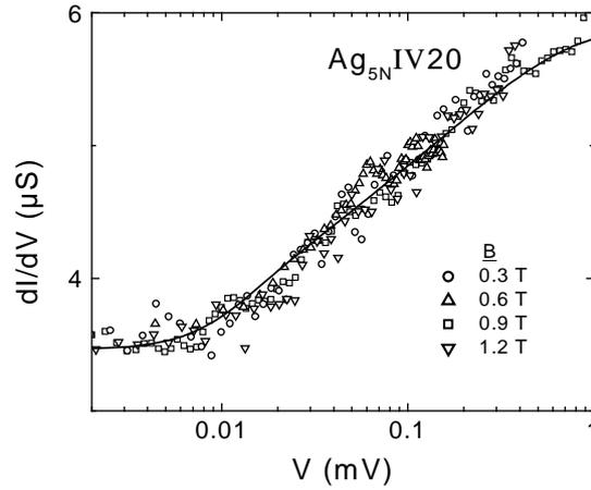
Figure 23: Symbols: Measured Coulomb blockade signal, for the sample Ag<sub>5N</sub>IV20 when the wire is at equilibrium for different applied magnetic fields. Solid line: Fit of the data using Coulomb blockade theory and the parameters summarized in Table 6. The magnetic field has no visible effect.
