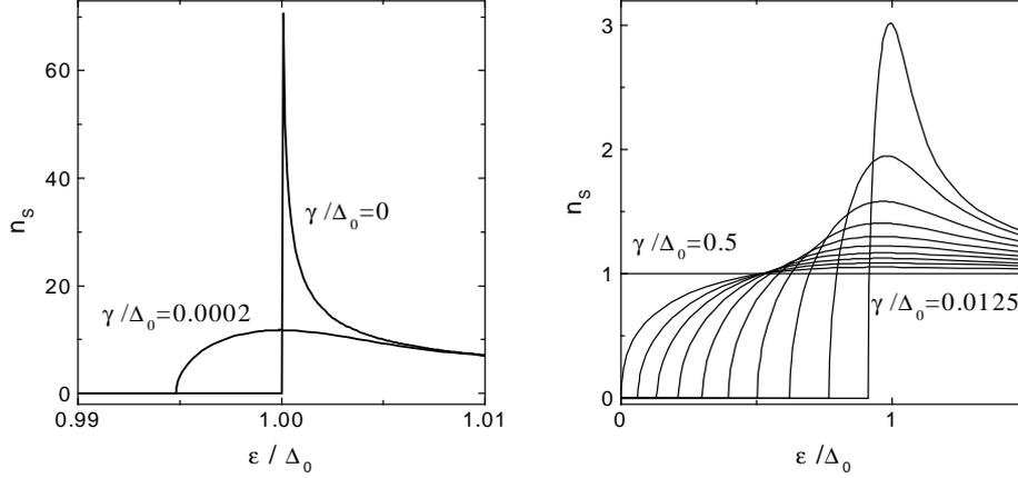
Figure 2: Theoretical predictions for the DOS in a superconductor versus reduced energy for several values of the depairing energy  $\gamma$ . Left panel:  $\gamma = 0$  and  $0.0002$ . Right panel: from right to left:  $\gamma = 0.0125$ , and  $0.05$  to  $0.5$  by steps of  $0.05$  in units of  $\Delta_0$ , the order parameter when  $\gamma = 0$ .
