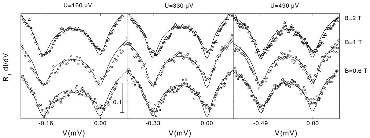
Figure 18: Symbols: Differential conductance  $dI/dV$  of a tunnel junction between a resistive probe electrode and an aluminum wire as a function of the bias voltage  $U$  across the wire and the applied magnetic field  $B$ . The curves have been vertically offset for clarity. At all the voltages,  $dI/dV$  does not depend on the magnetic field, proving the absence of KIM interaction. Solid lines: Fit with the parameters of Table 3, which are the same for all values of the magnetic field.
