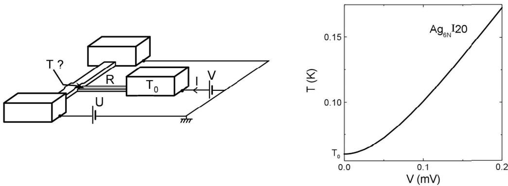
Figure 25: Left: Schematic of the circuit measurement. Electrons of the probe electrode are heated up by the measurement current only by their diffusive flow to the contact at  $T_0$ . Right: Electronic temperature  $T$  in the probe electrode at the junction position dependence on the voltage  $V$  for the Sample  $\text{Ag}_{6\text{N}}\text{I20}$  where  $R_p = 1.65 \text{ k}\Omega$  and  $R_T = 103 \text{ k}\Omega$ .
