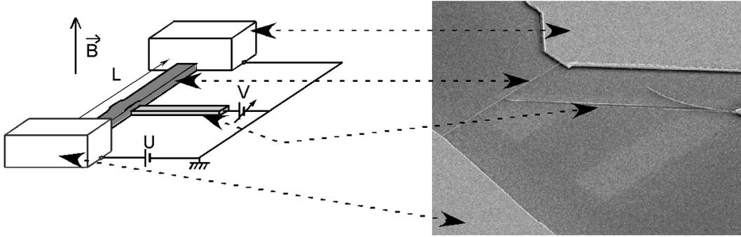
Figure 6: Left: Schematic of the circuit. A diffusive wire of length  $L$  is connected to two reservoirs biased at different potentials  $0$  and  $U$ . A long and narrow superconducting probe electrode forms a tunnel junction with the wire in its middle. Right: Micrograph of a sample seen at an angle with arrows related to the corresponding elements on the schematic.
