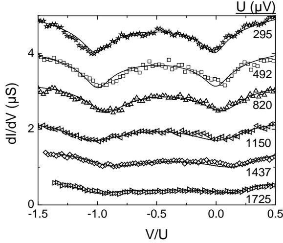
Figure 20: Symbols: Measured bias voltage  $U$  dependence of the differential conductance of a tunnel junction between a normal resistive tunnel junction and an aluminum wire in an applied magnetic field  $B = 2$  T. The data have been vertically offset and  $V$  normalized to  $U$  for clarity. Lines: Fits with the parameters summarized in Table 3.
