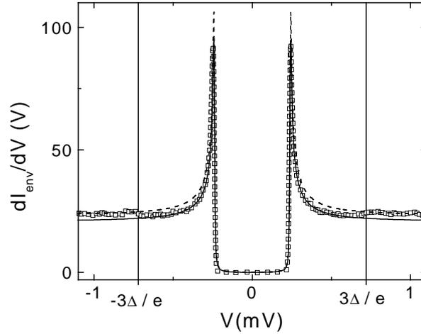
Figure 22: Symbols: Differential conductance  $dI_{env}/dV(V)$  of a normal-superconducting tunnel junction embedded in a superconducting environment. Due to Coulomb blockade of tunneling of quasiparticles, a rounded step appears at the voltages  $\pm 3\Delta/e$ . Between these voltages, the curve is fit using a BCS density of states in the superconducting probe (dashed line) with a renormalized tunnel conductance (solid line).
