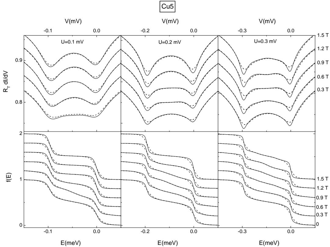
Figure 21: Calculated differential conductance  $dI/dV$  and energy distribution functions  $f(E)$  with the parameters found to account for the data of Cu5 (see Table 3) taking into account heating of the reservoirs (dashed line) or neglecting it (solid lines).
