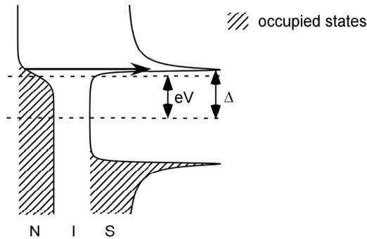
Figure 11: Principle of electron cooling effect in a normal superconducting tunnel junction. When the junction is biased just below the gap of the superconducting part, only hot quasiparticles from the normal part can tunnel, resulting in an effective cooling of the normal part.
