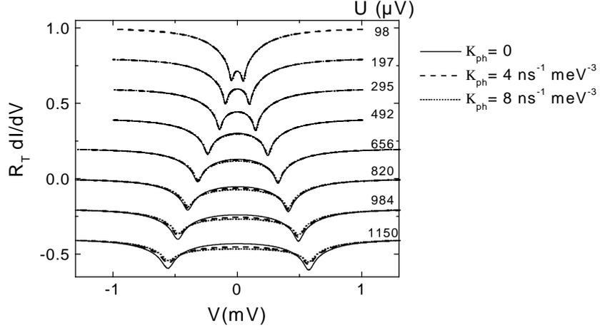
Figure 19: Influence of the electron-phonon interaction on the differential conductance  $dI/dV$  of the tunnel junction of the sample Al5 for different wire bias voltage  $U$ . Solid lines:  $\kappa_{ph} = 0$ . Dashed lines:  $\kappa_{ph} = 0.4 \text{ ns}^{-1} \text{ meV}^{-3}$ . Dotted lines:  $\kappa_{ph} = 0.8 \text{ ns}^{-1} \text{ meV}^{-3}$  (see other parameters in Table 3). Electron-phonon interaction has a non-negligible effect only for the larger wire bias voltage.
