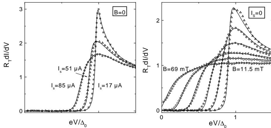
Figure 13: Normalized differential conductance of the probe tunnel junction: Left: at  $B = 0$ , as a function of the supercurrent  $I_s$ . Right: at  $I_s = 0$ , as a function of the magnetic field  $B$ . The solid lines are the best fits of the data.
