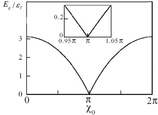
Figure 3: Energy gap  $E_g$  in units of the Thouless energy versus the phase difference  $\chi_0$  between the two superconducting contacts (from [5]). The inset shows the linear dependence of  $E_g$  near  $\chi_0 = \pi$ .
