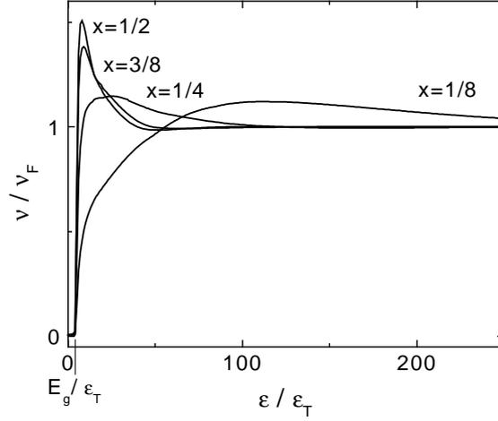
Figure 4: Density of states along a normal wire connected to two superconducting pads at the same phase. A minigap appears in the DOS. Its value does not depend on position.
