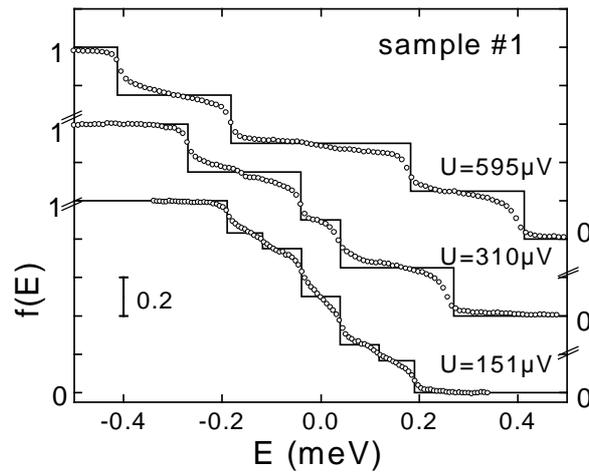
Figure 14: Energy distribution functions in the middle of the wire of sample 1, when the reservoirs are in the superconducting states and voltage biased at  $U$ . Symbols are experimental data; solid lines are the expectation of a simplified theory taking only into account multiple Andreev reflections.
