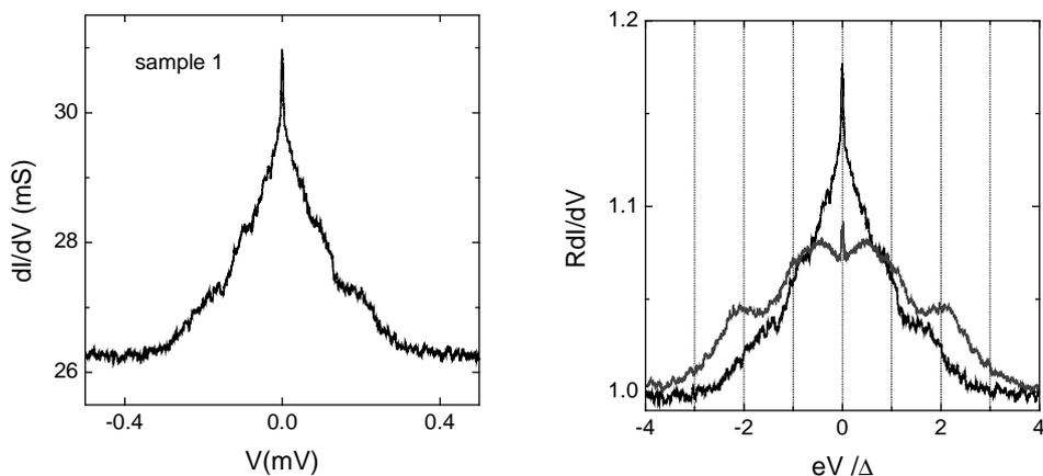
Figure 19: Left panel: Measured differential conductance  $dI/dV$  of the normal wire in sample 1. The conductance of the wire shows a step-like behavior as a function of the voltage. Right panel: Differential conductance, normalized to the conductance at large voltage  $1/R$ , versus voltage, normalized to the gap voltage of the superconducting pads  $\Delta$ , for sample 1 (black line) and 2 (gray line).
