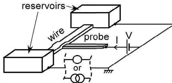
The metallic wire under investigation is connected to large pads, and it can be current biased or driven out-of-equilibrium by a voltage. A probe electrode forms a tunnel junction with the wire. Assuming that the density of states and the filling factors of the probe electrode are known, the density or filling of the states in the wire at the position of the junction can be inferred from the differential conductance  $dI/dV(V)$  of the tunnel junction.
