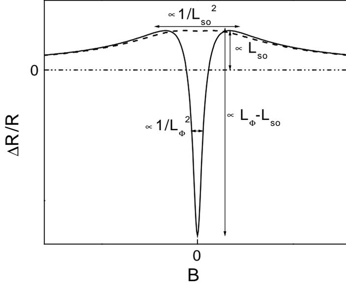
Figure 2: Generic magnetoresistance curves calculated with Eq. (4). The amplitudes and characteristic fields are given by the spin-orbit length  $L_{so}$  and the phase coherence length  $L_\phi$ . Solid line:  $L_\phi = 6L_{so}$ , dashed line: Same  $L_{so}$  and  $L_\phi = L_{so}$ .
