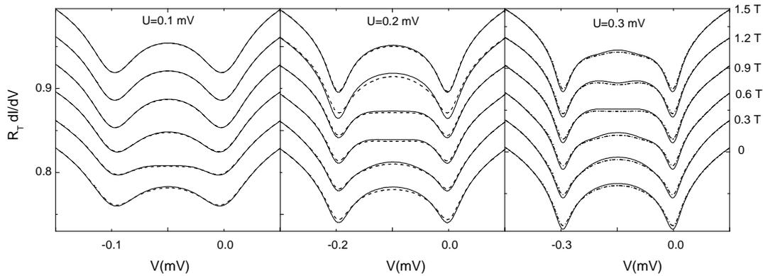
Figure 17: Calculated differential conductance  $dI/dV$  for different applied magnetic field with the fixed parameters for KIM interaction:  $c_{imp}/(v_F h) = 5$ ,  $g = 2.3$  and  $D = 1$  eV and the different couple of parameters  $(T_K, v_F J_0) = (100 \text{ mK}, 0.08)$  for the solid lines and  $(T_K, v_F J_0) = (300 \text{ mK}, 0.1)$  for the dashed lines. The curves have been vertically offset for clarity.
