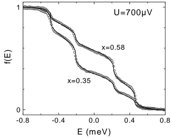
Figure 7: Symbols: Distribution functions measured at two positions in a 5  $\mu\text{m}$ -long silver wire, connected at both ends ( $x = 0$  and  $x = 1$ ) to superconducting electrodes biased at the potential 0 and 700  $\mu\text{V}$ . Solid lines: Solution of the Boltzmann equation accounting for the Andreev reflections at the reservoirs and electron-electron interactions within the wire.
