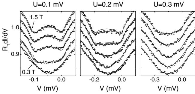
FIG. 3. Magnetic field effect in sample No. 1: differential conductance  $dI/dV(V)$  at  $U = 0.1, 0.2$  and  $0.3$  mV, for  $B$  ranging (from bottom to top) from  $0.3$  to  $1.5$  T by steps of  $0.3$  T. Successive curves have been vertically offset by steps of  $0.033$ , for clarity.
