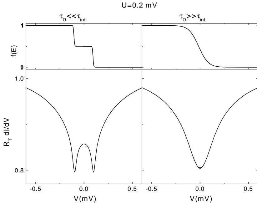
Figure 7: Top: Calculated distribution functions in the middle of an out-of-equilibrium wire in two extreme cases:  $\tau_n \ll \tau_{int}$  (left) and  $\tau_n \gg \tau_{int}$  (right). Bottom: Corresponding calculated differential conductance  $dI/dV$  of a tunnel junction formed between the wire and a resistive probe. The curve  $dI/dV$  shows a double dip when only little interaction occurs while electrons travel through the wire, and a broad single dip when electrons thermalize.
