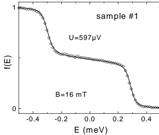
Figure 15: Energy distribution function in the middle of the wire of sample 1, when the reservoirs are in the normal state and voltage biased at  $U = 597 \mu V$ .
