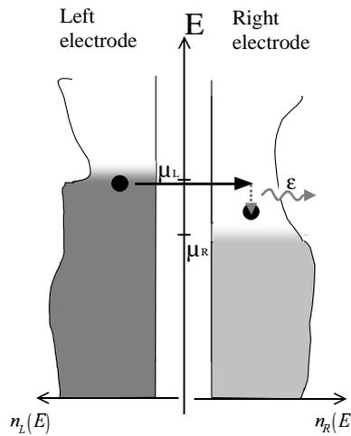
Figure 2: Tunneling process through a junction when the junction is voltage biased:  $eV = \mu_L - \mu_R$ . The current through the junction depends on the density of states in the electrodes  $n_L$  and  $n_R$ , the filling of these states  $f_L$  and  $f_R$ , and the probability  $P(\varepsilon, T)$  that the energy  $\varepsilon$  is released to the electromagnetic environment.
