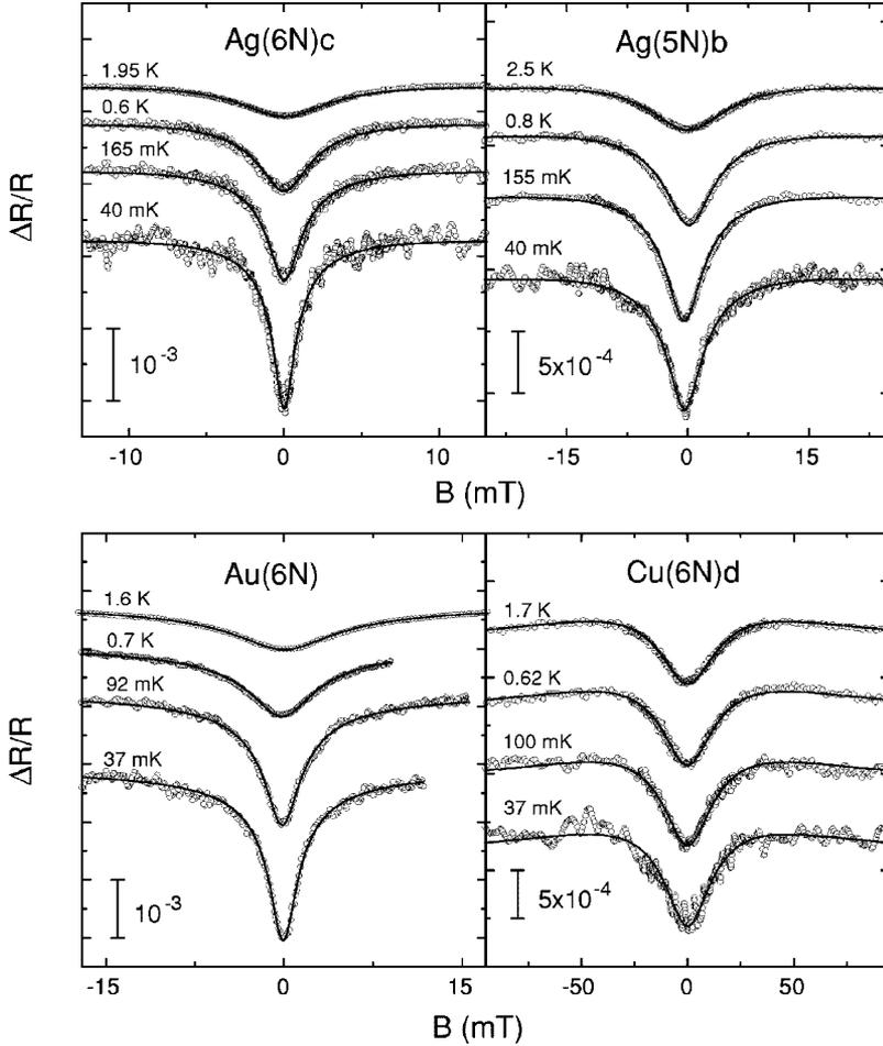
FIG. 2. Magnetoresistance data (symbols) and fits to Eq. (1) (solid lines). Top panels are measurements of two silver samples made of source materials of nominal purity 6N (99.9999%, top left panel) and 5N (99.999%, top right panel). Bottom panels display data measured on gold (bottom left panel) and copper (bottom right panel) samples made of 6N nominal purity source materials. The curves are offset vertically for clarity.
