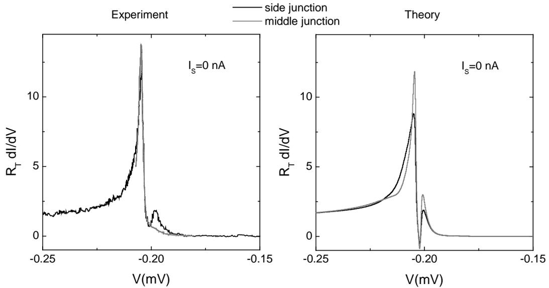
Figure 11: Left: Normalized differential conductance of the two tunnel junctions when the phase difference  $\chi_0$  between the two superconducting pads is zero. Right: Theoretical predictions using the DOS calculated in Section 11.2.1.
