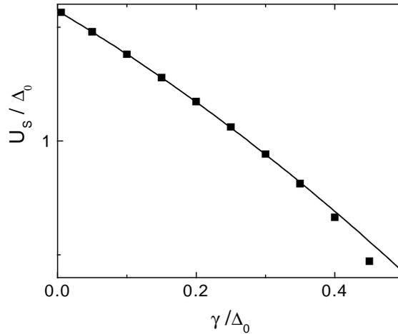
Figure 6: Symbols: Numerical calculation of the pair energy  $U_s$  in units of  $\Delta_0$  versus the depairing energy. Solid lines: Approximate expression  $U_s(\gamma)/\Delta_0 \approx \pi/2 - 1.8 \gamma/\Delta_0 - 1.0 (\gamma/\Delta_0)^2$ .
