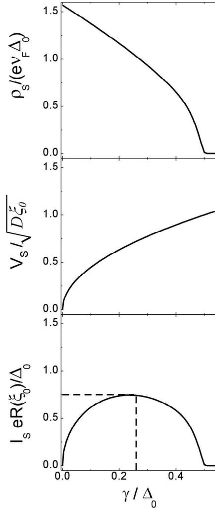
Figure 7: The normalized supercurrent (bottom panel) through a wire is proportional to a density of charge in the superconducting state  $\rho_s$  (upper panel) times the superfluid velocity  $V_s$  (middle panel). The supercurrent versus the depairing energy reaches a maximum corresponding to the critical current at  $\gamma/\Delta_0 = 0.238$ , leading to  $I_c \approx 0.75 \Delta_0 / (eR(\xi_0))$ .
