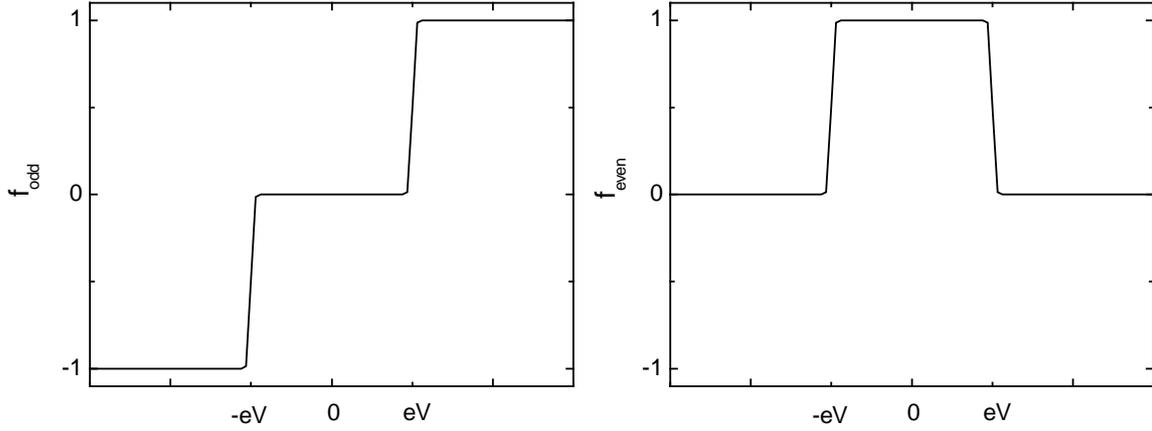
Figure 2: Odd and even part of the energy distribution function used in the theory of non-equilibrium superconductivity, in the case where the system is a reservoir at a potential  $V$ .
