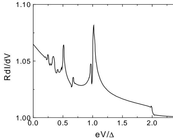
Figure 21: Predicted differential conductance of a normal wire connected to two superconducting reservoirs of gap  $\Delta$ . The length of the normal wire is  $9L_\Delta = 9\sqrt{\hbar D}/\Delta$  with  $D$  the diffusion constant of the normal wire. Peaks appear in the differential conductance at energies equal to submultiple of twice the gap.
