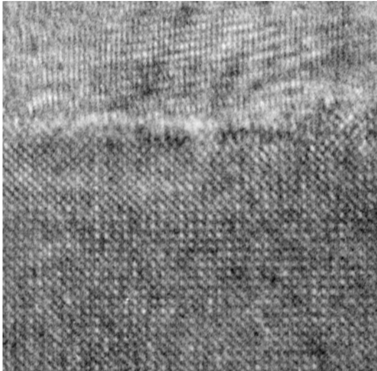
Figure 7.1: HRTEM image of a LSMO/STO/Co 84 Cr 16 trilayer (Al1689). MnO 2 columns in the lower La 0.7 Sr 0.3 MnO 3 layer are expanded to the 3.905Å STO lattice spacing. Picture by Patricia Prod'homme.
