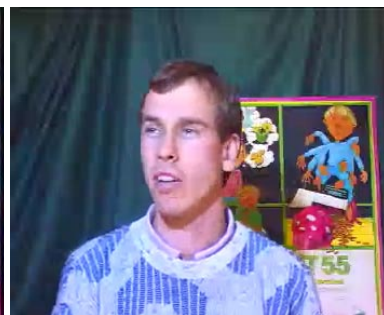
(c) Codage H26L VM 8 R=52 Kb/s PSNR_{avant-plan}=26,9
