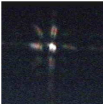
Figure 6: An example of laboratory results with two artificial stars in the ZOF. The two white peaks are visible, together with colored dispersed peaks at the edge of ZOF. The image has been printed at \gamma=0.25 for clarity.
