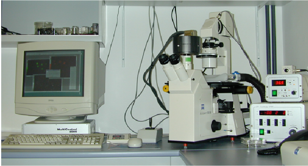
Figure 5.1: Imaging workstation: an inverted microscope coupled to the camera (on the top) with automated shutters and an incubation chamber connected to the controlled system on the right.
