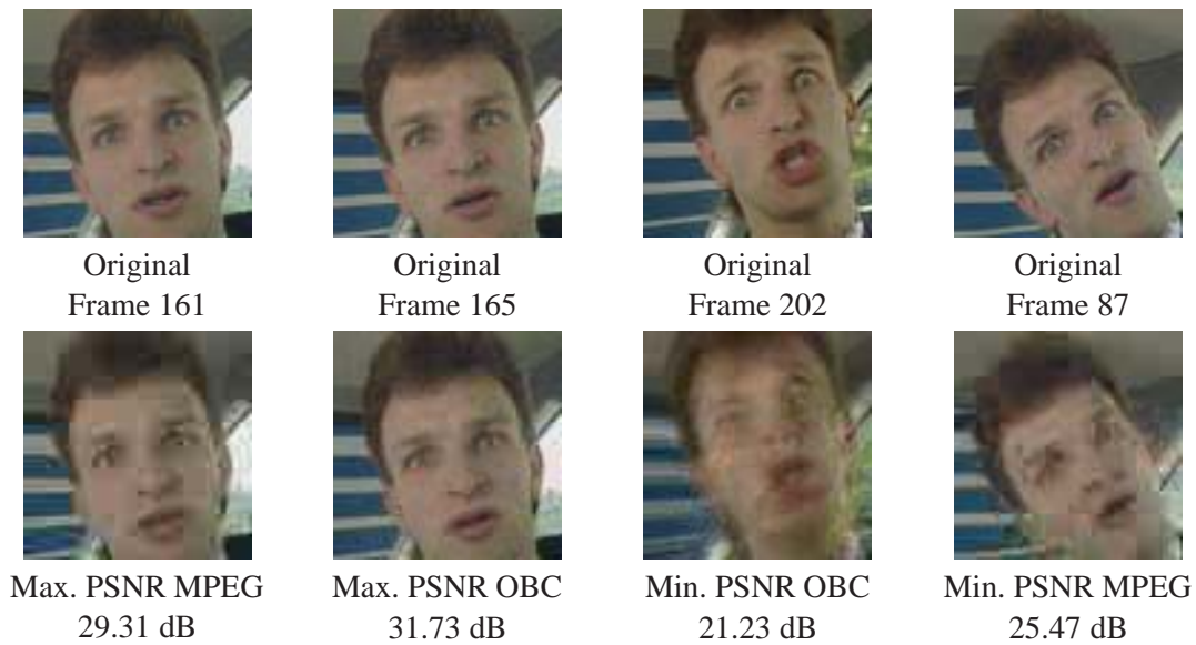
FIG. 8.7: Example frames from sequence CARPHONE showing the coding artifacts, illustrated by the best (maximum PSNR) and worst (minimum PSNR) reconstruction : MPEG encoding with P : B : I quantizer scales of 24 : 22 : 19 (avg. PSNR 27.58 ; CR 113.75 : 1), and for OBC with 40 basis images and quality parameter 55 (avg. PSNR 26.92 ; CR 102.90 : 1).
