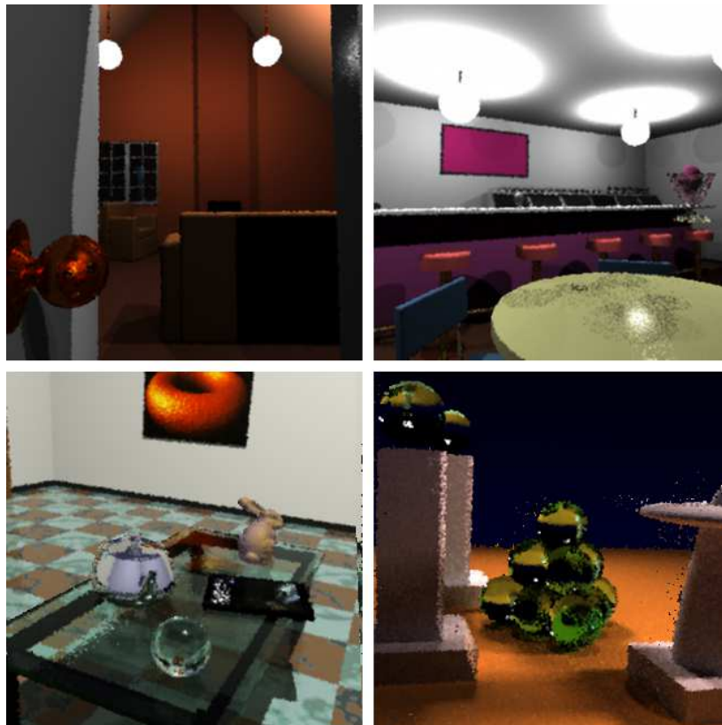
Fig. 8. Some example images captured from interactive sessions. Some approximation artifacts are visible but the overall image quality is good. All scenes are ray traced except the lower right which is path traced. In the upper right image we have just moved the ice cream glass and you can see its shadow in the process of being updated on the table top.
