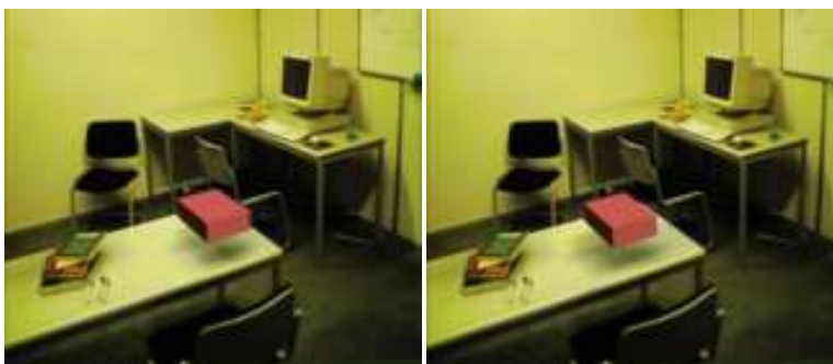
Fig. 6. (a) The complete CAR rendering using the RVI texture polygons for display, including the CG object (b) The CG object has moved to the left: the update takes 2.5 seconds.
