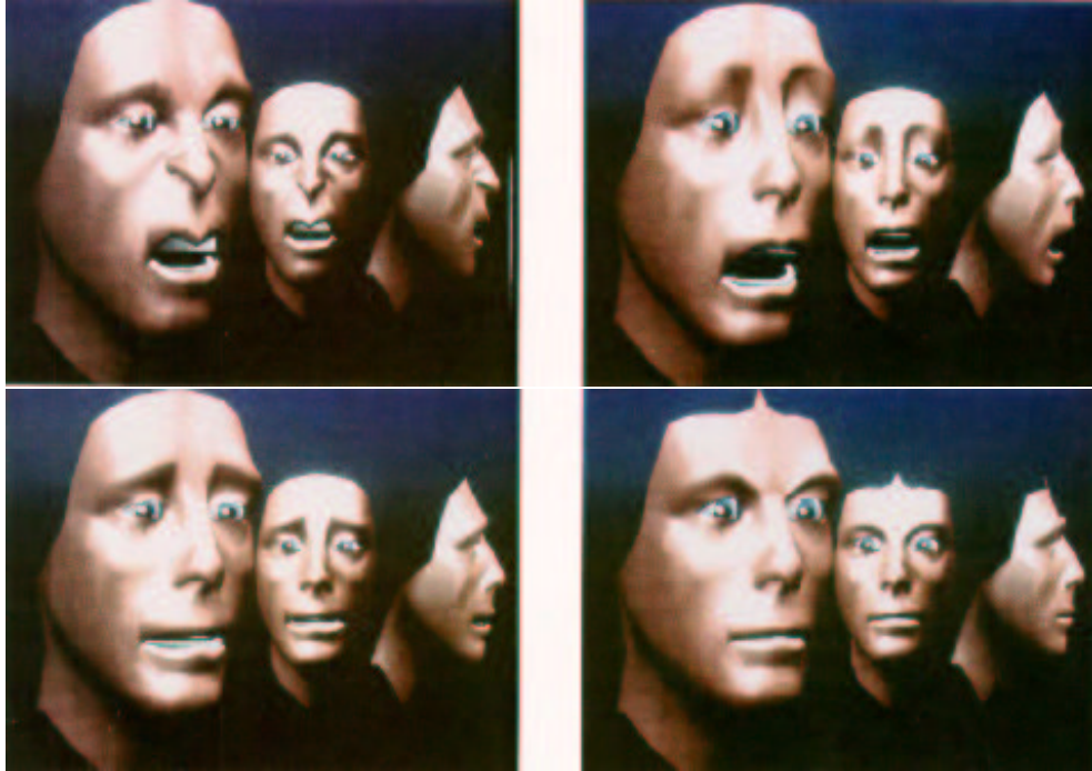
Figure 2.2: Facial (skin) modeling and animation by K. Waters using mass-spring models. Taken from [TERZOPOULOS AND WATERS, 1990].
