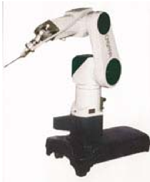
Figure 2.4: The CASPAR robot
