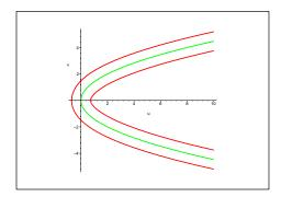
Figure 4.4.23: A parabola and its 0.5-generalised offset
