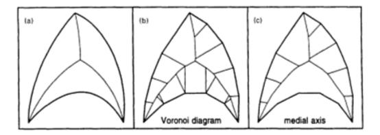
Figure 2.3.2: The internal part of the Voronoi diagram and the medial axis are identical for the exact boundary while they differ for the approximate boundary (taken from [RF99a])
