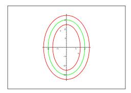
Figure 4.4.13: An ellipse and its 0.5—generalised offset
