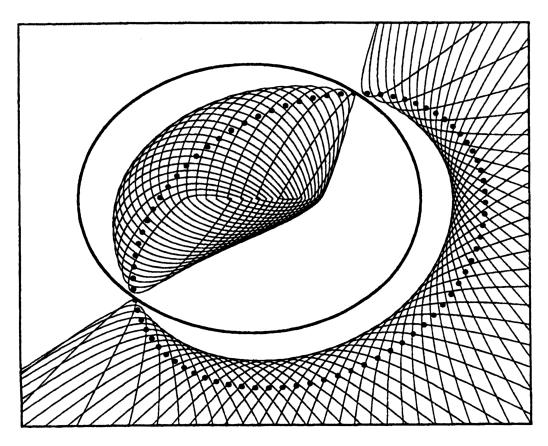
Figure 2.3.3: The bisector of two curves as the envelope of a family of point/curve bisectors (taken from  $[\mathrm{FR}98\mathrm{b}])$
