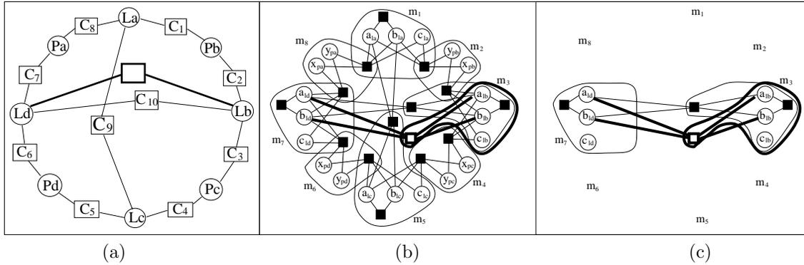
Figure 9.4: Failure of GPDOF in presence of a redundant parallelism constraint. (a) The parallelism constraint is redundant to the parallelism  $C_{10}$  (in the constraint graph). (b) The enriched equation graph with the corresponding additional equation (white rectangle) and two additional r-methods (only one is represented). (c) After having removed all possible free r-methods and submethods, GPDOF is stuck because the redundant equation prevents r-method  $m_3$  from being free.
