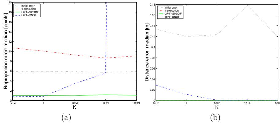
Figure 11.7: Optimization results as a function of increasing  $K$  factor; (a) Median reprojection error; (b) Median distance error. Note that after at least one GPDOF execution the distance constraints are respected exactly, so the curves corresponding to the model after 1 GPDOF execution and after the GPDOF-based optimization are identical to the  $x$ -axis.
