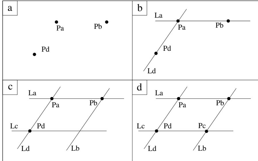
Figure 8.3: Execution of r-methods in the plan ( $m_1, m_7, m_3, m_5, m_4$ ). (a) The input parameters (i.e., coordinates of  $\mathbf{P}_a$ ,  $\mathbf{P}_b$  and  $\mathbf{P}_d$ ) are replaced by their current value. (b)  $m_1$  and  $m_7$  place lines  $\mathbf{L}_a$  and  $\mathbf{L}_d$  resp. (c)  $m_3$  and  $m_5$  place  $\mathbf{L}_b$  and  $\mathbf{L}_c$  resp. (d) Finally,  $m_4$  places point  $\mathbf{P}_c$ .
