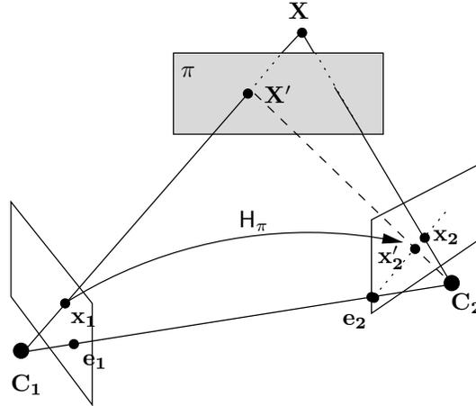
Figure 2.3: The concept of plane induced parallax. Point  $\mathbf{x}'_2 = H_\pi \mathbf{x}_1$  is the image of point  $\mathbf{X}'$  lying on the intersection of ray  $C_1 \mathbf{x}_1$  and plane  $\pi$ . It is collinear with the point  $\mathbf{x}_2$  being the true image of point  $\mathbf{X}$  and the epipole  $\mathbf{e}_2$ . The vector  $\mathbf{x}_2 \mathbf{x}'_2$  is the parallax relative to homography  $H_\pi$ .
