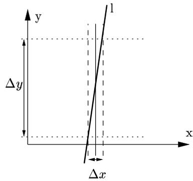
Figure C.1: Well-conditioned and bad conditioned computations. Based on the represented line equation, the computation of the coordinate  $y$  using values of  $x$  is much more sensitive to noise than the computation of coordinate  $x$  using values of  $y$ .
