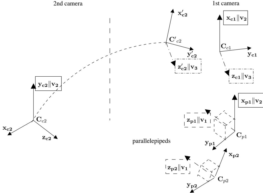
Figure 7.3: Experimental setup for tests on synthetic data: one camera is static ( $C_{c1}$ ) and the second one moving (from position  $C_{c2}$  to  $C'_{c2}$ ). They are watching two parallelepipeds (at  $C_{p1}$  and  $C_{p2}$ ). Parallel directions are drawn using the same line style and label  $v_{i \in \{1,2,3\}}$ .
