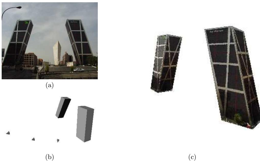
Figure 7.18: Kio towers in Madrid: (a) The original image; (b), (c) Screen-shots of the reconstructed model.
