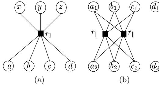
Figure 8.5: Representation of dependencies between object coordinates induced by constraints. (a) a point-plane incidence constraint (1 dof) is represented by the equation:  $ax+by+cz+d=0$  relating all the variables of both objects. (b) a plane-plane parallelism constraint (2 dofs) is represented by equation  $(a_1, b_1, c_1) \sim (a_2, b_2, c_2)$  relating only the variables representing both plane normals.
