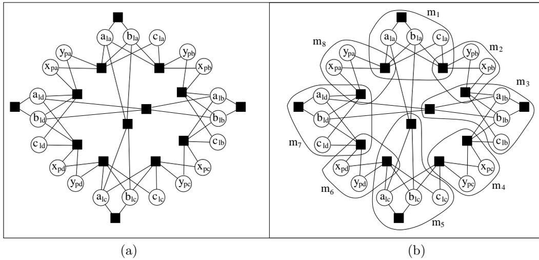
Figure 8.2: (a) The equation graph of the 2D scene. Variables are represented by circles and equations are represented by black rectangles. An equation implying only the  $a$  and  $b$  coordinates of a line has the form  $a^2 + b^2 = 1$  and allows a unique representation of a line. (b) The enriched equation graph. An  $r$ -method is represented by a hyper-arc including its equations and its output variables. Only eight of the sixteen possible  $r$ -methods are depicted for the sake of clarity.
