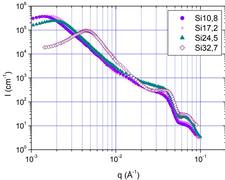
Figure III-24. Spectres SAXS des nanocomposites fortement chargés
