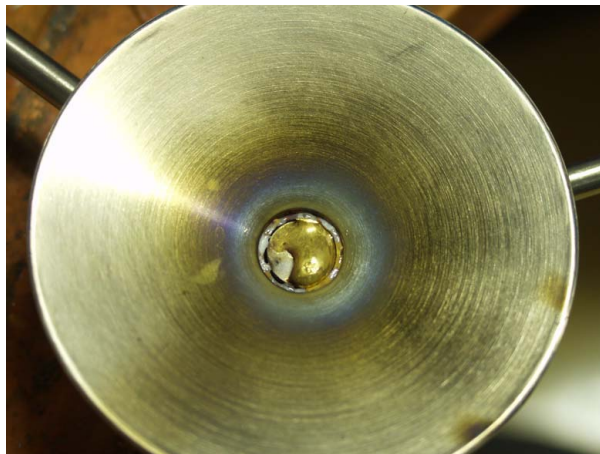
Figure 3.9: Example of target destroyed after melting. In the center we see the gold fused into a big drop, no more usable for francium production. The cone which surrounds the gold target is the extraction electrode.
