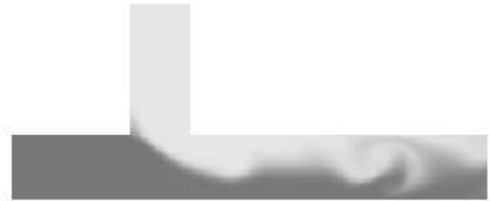
FIG. 4.4 – Instantaneous temperature fields in a 2D unsteady Tee junction at t = 12.2s (8 recirculation times) - non-physical temperature regions ( ie out of limits) are denoted by dark contours.
