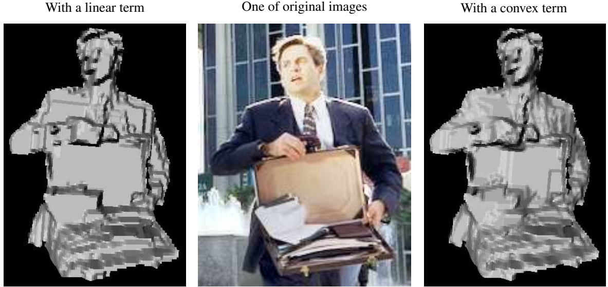
Fig. 2.27: Comparison between a linear and a convex smoothing term (influence on 3D results)
