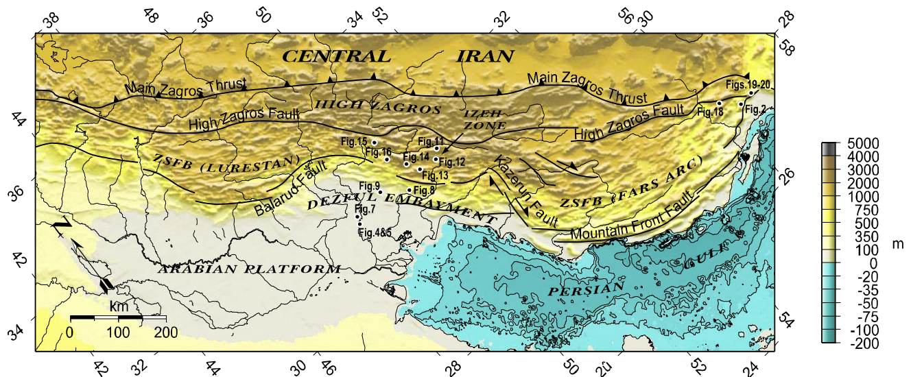
Fig. 1 Physical map (source: GEBCO data) and main structural features of the Zagros fold-thrust belt with location of the figures. See also appendix 5. ZSF: Zagros Simply Folded Belt.
