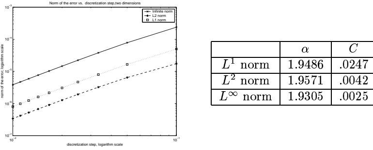
Figure 6.8: Convergence rate, two dimensional case, right hand side Dirac at zero, located at the center of the center cell, norm computed on a “regular zone”.
