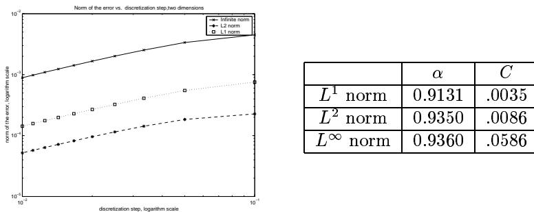
Figure 6.7: Convergence rate, two dimensional case, right hand side Dirac at zero, non symmetric discrete problem, norm computed on a “regular zone”.
