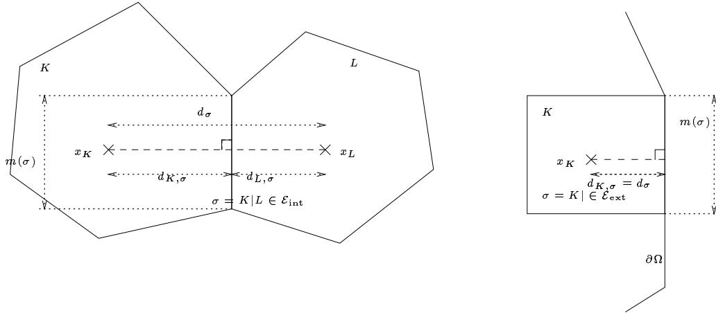
Figure 6.1: Notations for an admissible mesh
