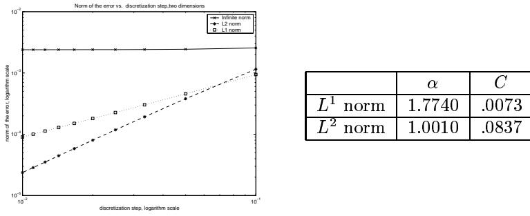
Figure 6.6: Convergence rate, two dimensional case, right hand side Dirac at zero, symmetric discrete problem.
