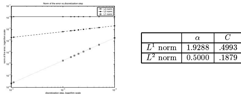
Figure 6.11: Convergence rate, three dimensional case, right hand side Dirac at zero, spherical case.
