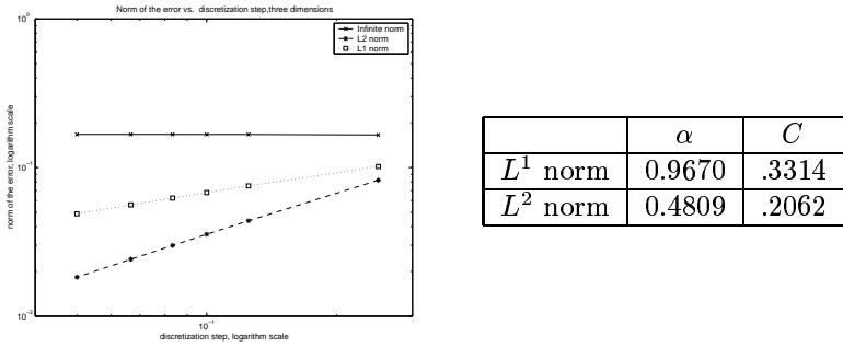
Figure 6.9: Convergence rate, three dimensional case, right hand side Dirac at zero, nonsymmetric discrete problem.
