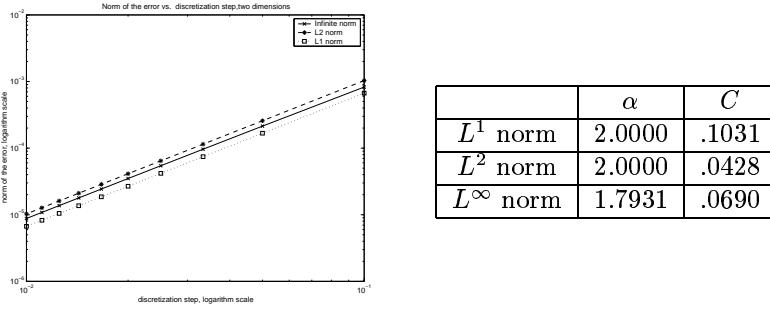
Figure 6.4: Convergence rate, two dimensional case, regular right hand side.
