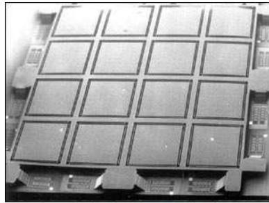
Photomicrograph showing early concept for a 3D scanning mirror, courtesy of Dr. Li Fan, OMM Director of MEMS Design
