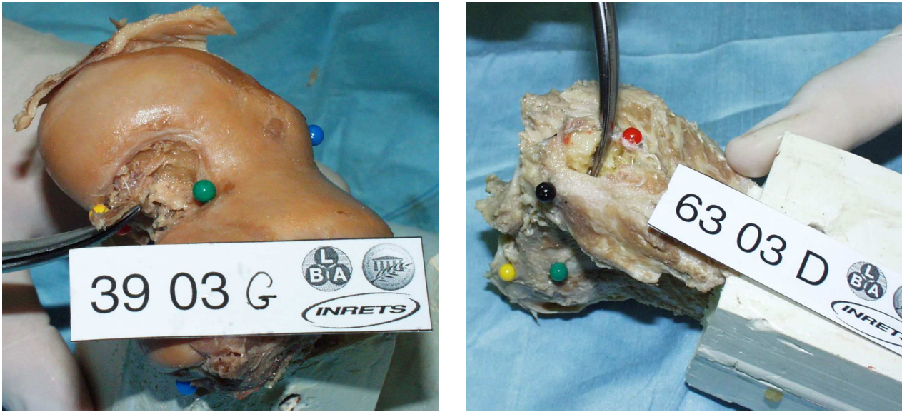
(a) Failure of the PCL femoral enthesis. (b) Failure of the LCL fibular enthesis.
