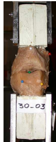
(b) Knee sample placed on the device in extension. The femur is at the top, the tibia is at the bottom, since it is more convenient with technical constraints.
