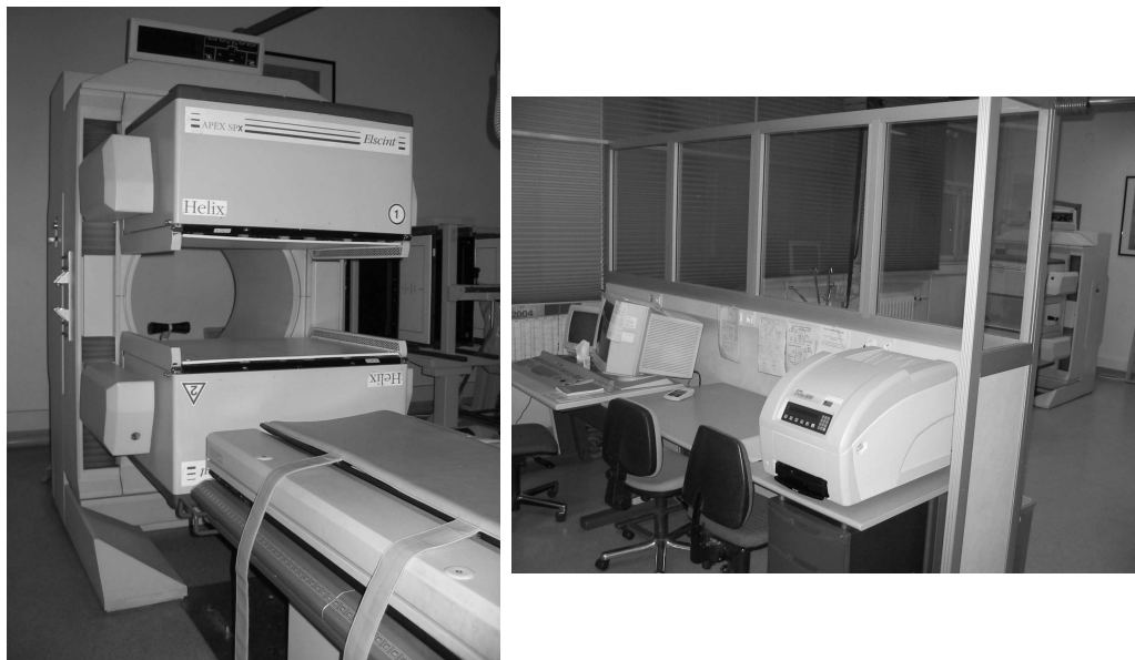
Figure 2.6: Photo of the gamma camera (left) used at our institute and the control room (right). The camera has two heads that are controlled by a motor (behind). The patient is placed on the bed with an additional support for his head. The camera heads are then positioned as close as possible to the patient's head. During acquisition, the camera heads rotate around the axis of the patient and the patient is asked to remain still. The acquisition procedure can be programmed and for brain SPECT, two 180 degrees rotations of the cameras are made with acquisitions (projections) at every 4 degrees for 10 seconds. The total acquisition time is about 20 minutes.
